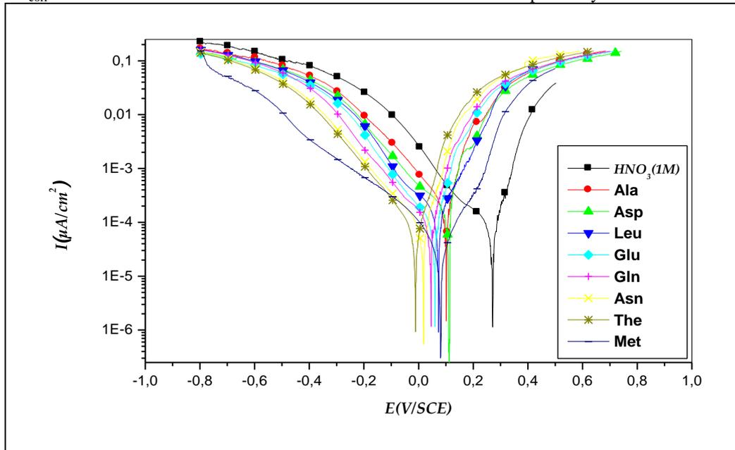
**Figure 2:** Polarization curves for copper in 1 mol L<sup>-1</sup>  $\text{HNO}_3$  solutions in the absence and presence of amino acids at  $10^{-3}$  M.
