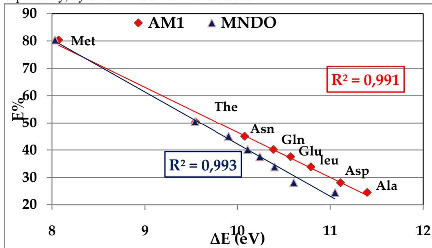
**Figure 4:** Correlation between energy gaps ( $\Delta E = E_{LUMO} - E_{HOMO}$ ) and efficiency of inhibition corrosion by the amino acids tested.
