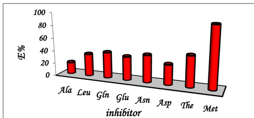
**Figure 3:** Variation of the efficiency of inhibition of corrosion of copper in 1M HNO<sub>3</sub> by amino acids at 10<sup>-3</sup>M.
