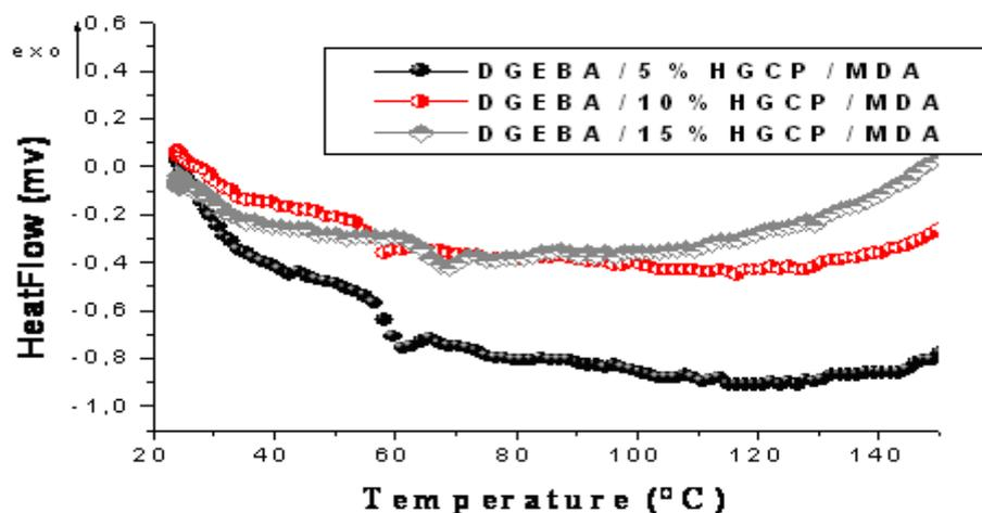
**Figure 5:** Comparison of DSC curves for formulations: [DGEBA/5%HGCP/MDA], [DGEBA/10%HGCP/MDA] and [DGEBA/15%HGCP/MDA].
