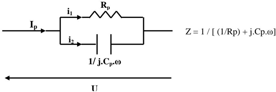
Figure 10: Parallel model of the equivalent impedance of material.
