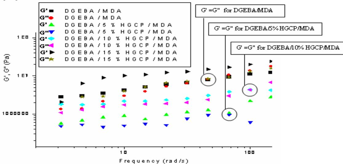
**Figure 7:** Elastic modulus  $G'$  and loss modulus  $G''$  as a function of frequency for (DGEBA/HGCP/MDA) blends. HGCP amounts are: 0%, 5%, 10% and 15%.
