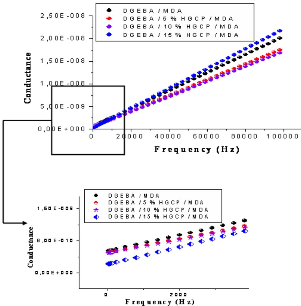
Figure 11: Conductance-Frequency characteristics of samples: [DGEBA/MDA], [DGEBA/5% HGCP/MDA], [DGEBA/ 10% HGCP/MDA] and [DGEBA/ 15% HGCP/MDA]
