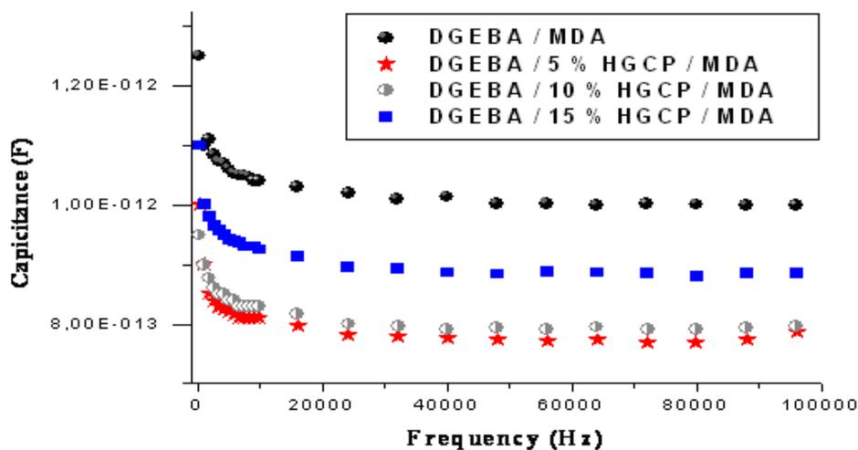
**Figure 9:** Capacitance-Frequency characteristics of samples: [DGEBA/MDA], [DGEBA/5%HGCP/MDA], [DGEBA/10%HGCP/MDA] and [DGEBA/15% HGCP/MDA]
