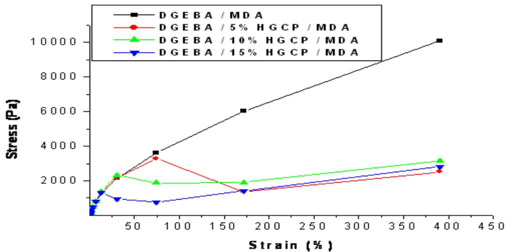
**Figure 8:** The stress-strain curves of DGEBA samples with different rates of HGCP (0% - 5% - 10% and 15%).
