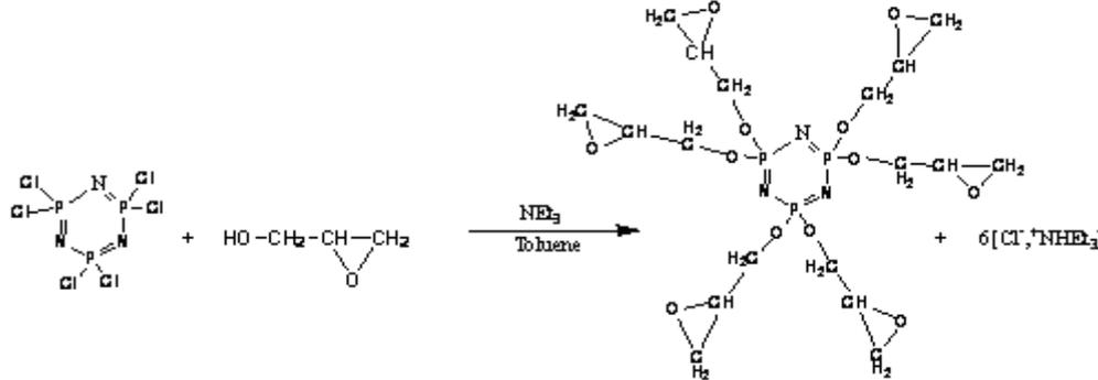
**Figure 1:** Synthesis of hexaglycidyl Cyclotriphosphazene (HGCP)
