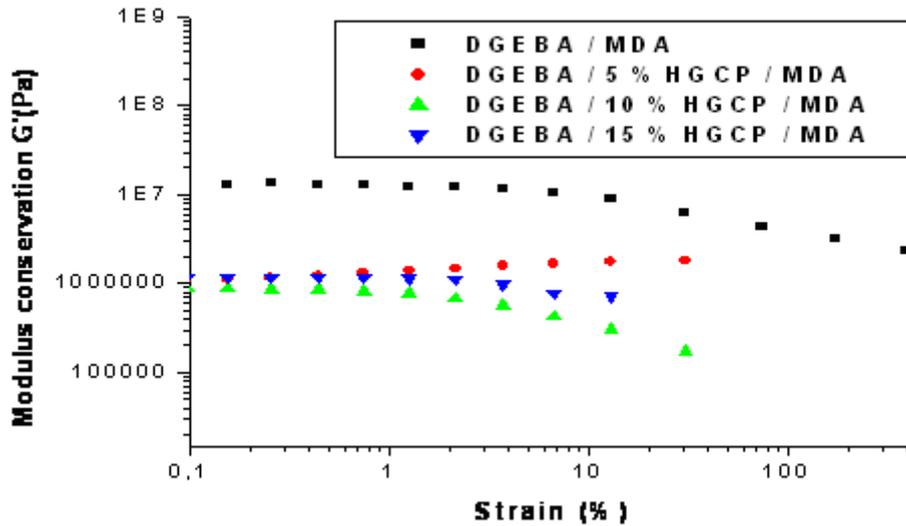
**Figure 6:** Modulus conservation  $G'$  as a function of strain for the DGEBA samples with different rates of HGCP (0%, 5%, 10% and 15%).
