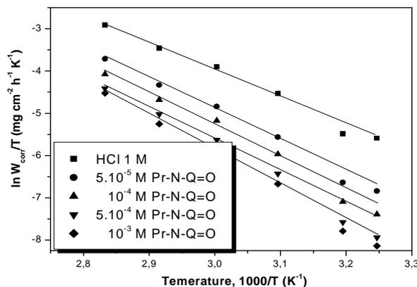
**Figure 6.** The relationship between  $\ln W_{corr}/T$  and  $1/T$  for mild steel at different concentrations of Pr-N-Q=O.
