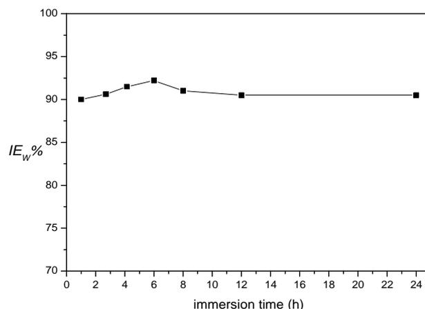
**Figure 3.** Variation of  $IE_w\%$  versus immersion time of mild steel in 1 M HCl without and with  $10^{-3} \text{ M}$  of Pr-N-Q=O at 308 K.
