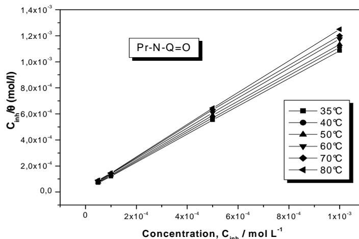
**Figure 7.** The relationship between  $C_{inh}/\theta$  and  $C_{inh}$  of Pr-N-Q=O at various temperatures.
