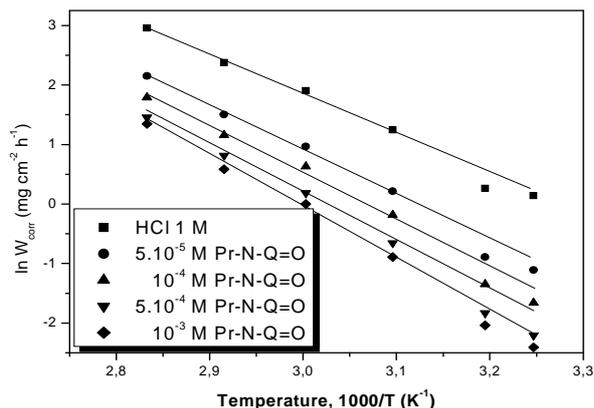
**Figure 5.** Arrhenius plots of mild steel in 1 M HCl at different concentrations of Pr-N-Q=O.
