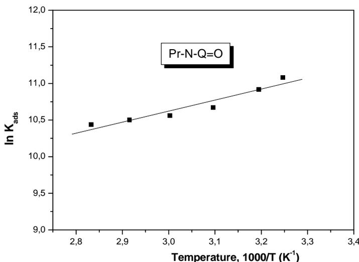
**Figure 8.** Van't Hoff plot for the mild steel/Pr-N-Q=O/1M HCl system
