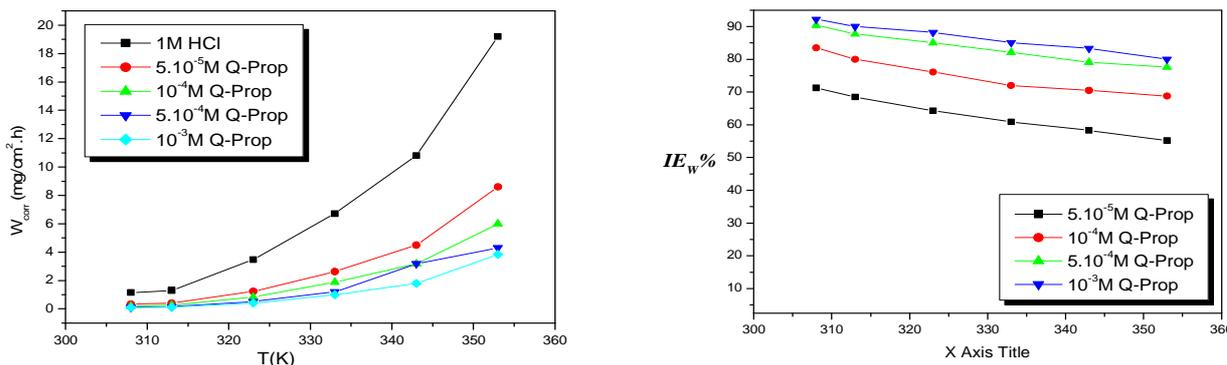
**Figure 4.** Variation of corrosion rate and inhibition efficiency with temperature for mild steel in 1 M HCl at different concentrations of Pr-N-Q=O.
