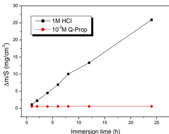
**Figure 2.** Weight loss versus immersion time of mild steel in 1 M HCl without and with  $10^{-3} \text{ M}$  of Pr-N-Q=O at 308 K.
