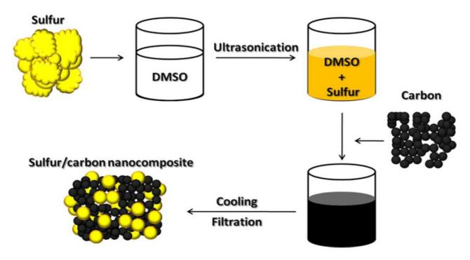
Fig. 1. Schematic of the solution processing for the preparation of sulfur/carbon [27]
