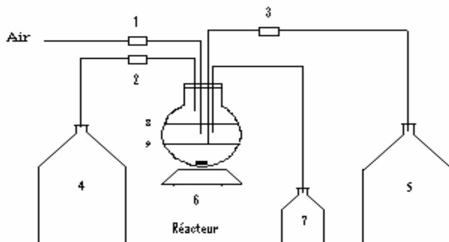
**Figure 1:** Schematic of the SBR process laboratory scale.
