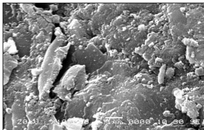
**Fig. 2** Scanning Electron Micrograph of Activated Carbon produced from bhagar seed husk
