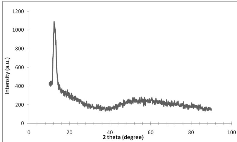
**Fig. 3** XRD Pattern of Activated Carbon produced from bhagar seed husk
