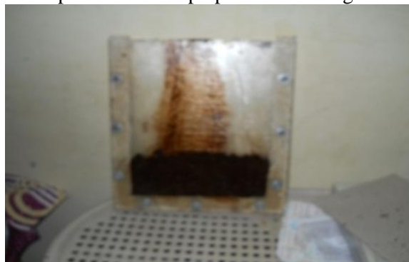
Figure 3: Mould for plate casting
