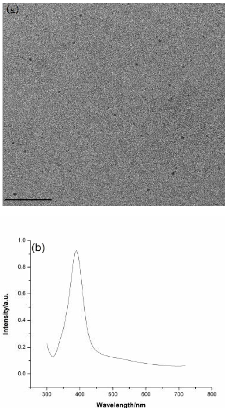
**Figure 1:** TEM (a) and UV-Vis spectrum (b) of synthesized nanosilver using Tollens' method (Black line=200 nm).
