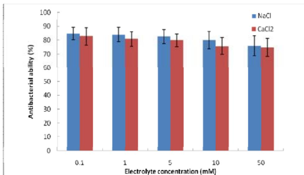
**Figure 3:** Antimicrobial properties of nanosilver in different electrolyte solutions.
