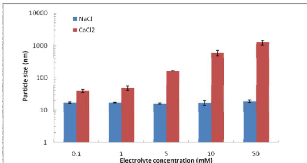
**Figure 4:** Particle size of nanosilver in different electrolyte solutions.
