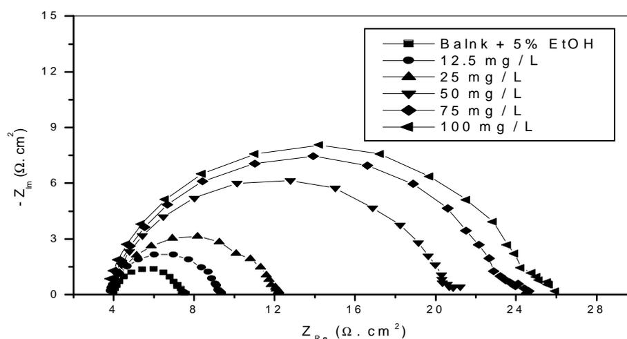
**Figure 2.** Complex plane plots for mild steel in the aggressive solution in the absence and in the presence of different concentrations of **LF-Ch** extract at 32°C.
