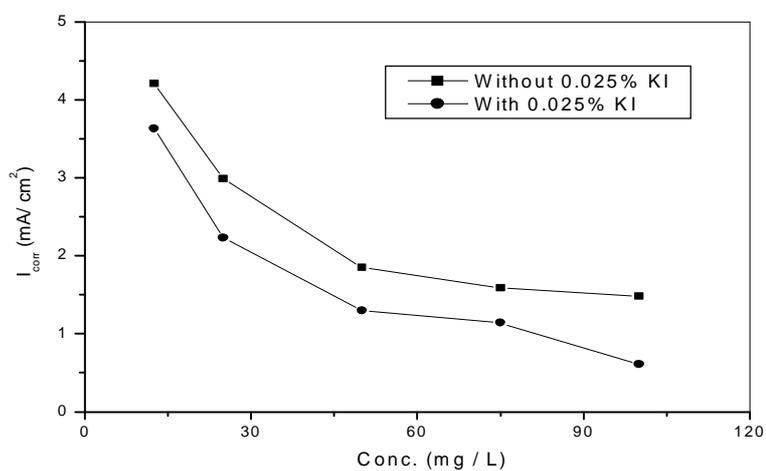
**Figure 5.**  $I_{corr}$  values in the absence and presence of 0.025% KI for different concentrations of LF-Ch extract.
