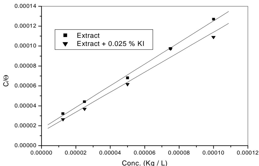
**Figure 8.** Langmuir adsorption isotherm of **LF-Ch** extract and **LF-Ch** extract+ KI on the mild steel surface
