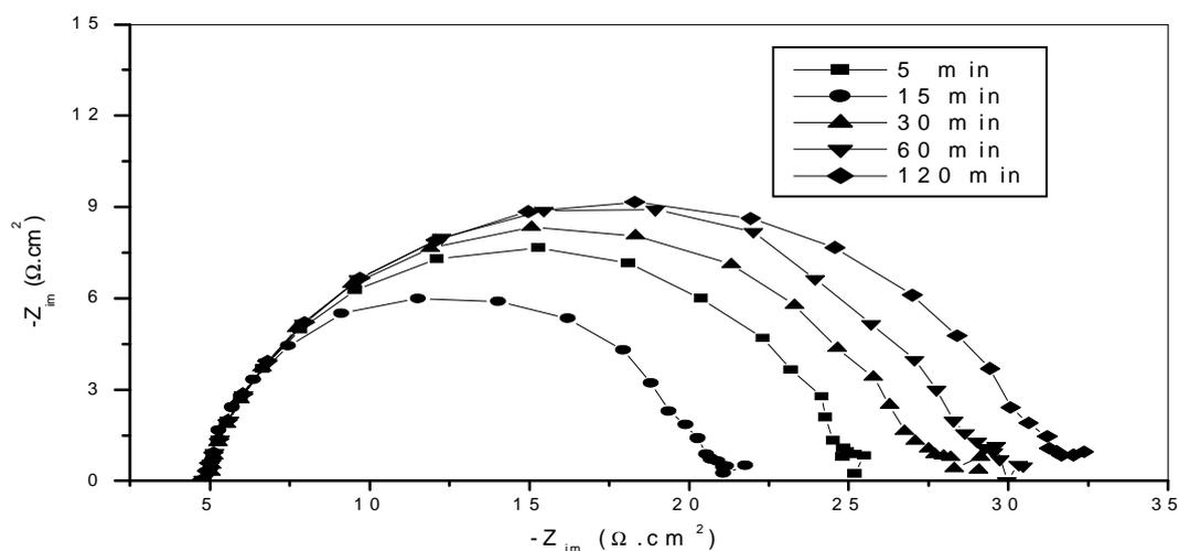
**Figure 7b.** Effect of immersion time on Nyquist plots of mild steel in 0.5M H<sub>2</sub>SO<sub>4</sub> + 5% EtOH in presence of 100 mg/L of **LF-Ch** extract.
