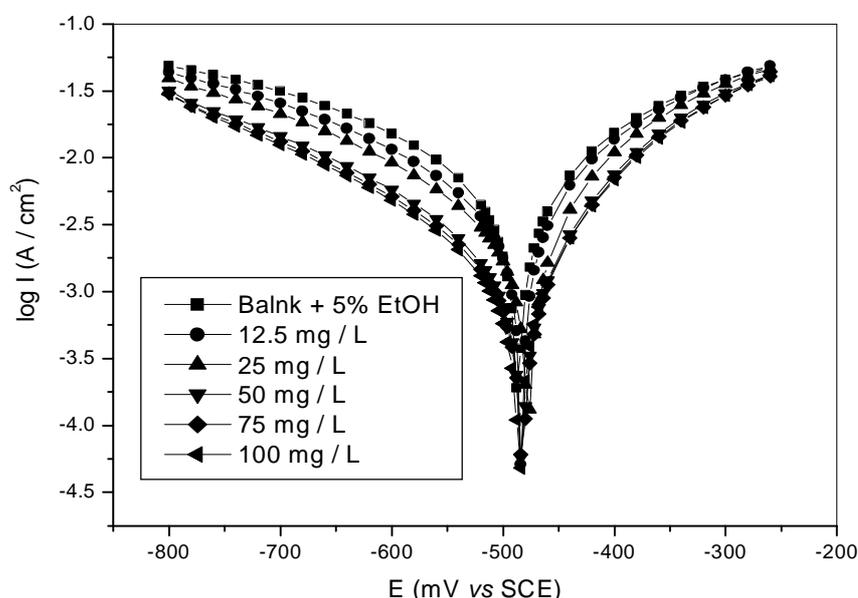
**Figure 1.** Potentiodynamic polarization curves for mild steel in 0.5 M  $\text{H}_2\text{SO}_4$  +5% EtOH containing different concentrations of **LF-Ch** extract at 32 °C.
