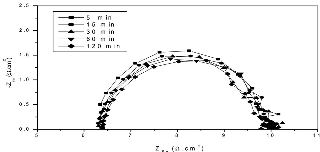
**Figure 7a.** Effect of immersion time on Nyquist plots of mild steel in 0.5M H<sub>2</sub>SO<sub>4</sub> + 5% EtOH in absence of **LF-Ch** extract.
