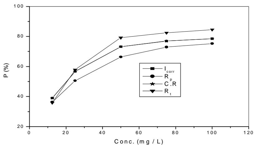
**Figure 4.** Inhibition efficiency vs inhibitor concentrations calculated by different methods
