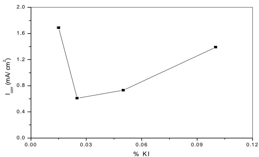
**Figure 6.** The plot of  $I_{corr}$  values vs. % KI for LF-Ch extract at 100 mg/L.
