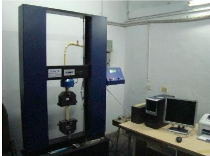
**Fig. 3:** Universal Testing Machine
