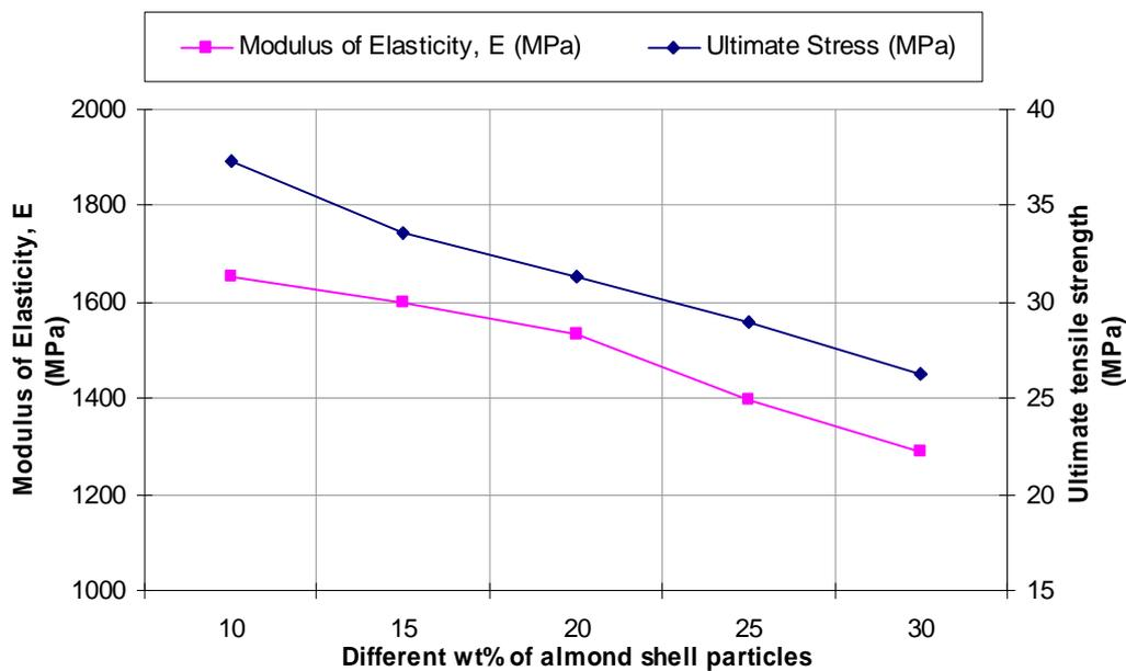
**Fig. 4:** Effect of different wt% of almond shell particles on ultimate tensile strength and modulus of elasticity.
