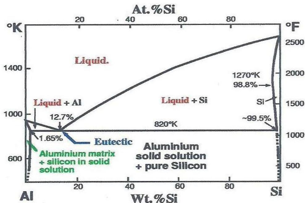
Figure 1: Al-Si cast alloy phase diagram [14]
