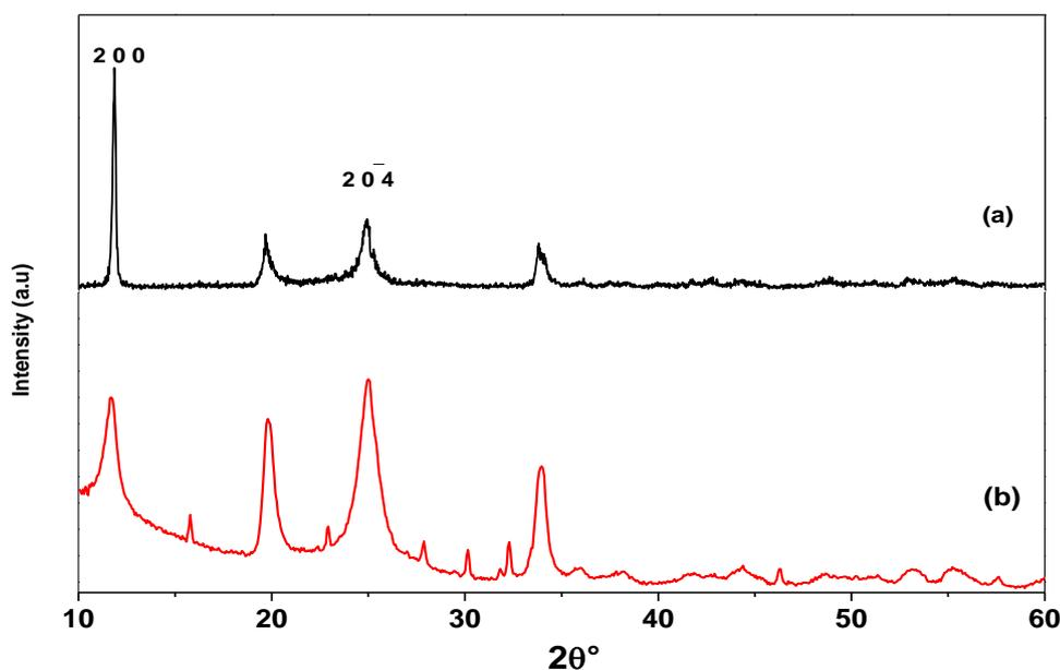
Fig. 1. X-ray powder diffraction of (a)  $\alpha$ -ZrP, and (b) Ag-ZrP
