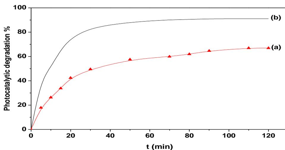
Fig. 4. Kinetics of photocatalytic degradation of MB on (a)  $\alpha$ -ZrP, and (b) Ag-ZrP. pH 3, V= 200 ml,  $m_{\text{cat}} = 100$  mg, [MB] = 100 ppm
