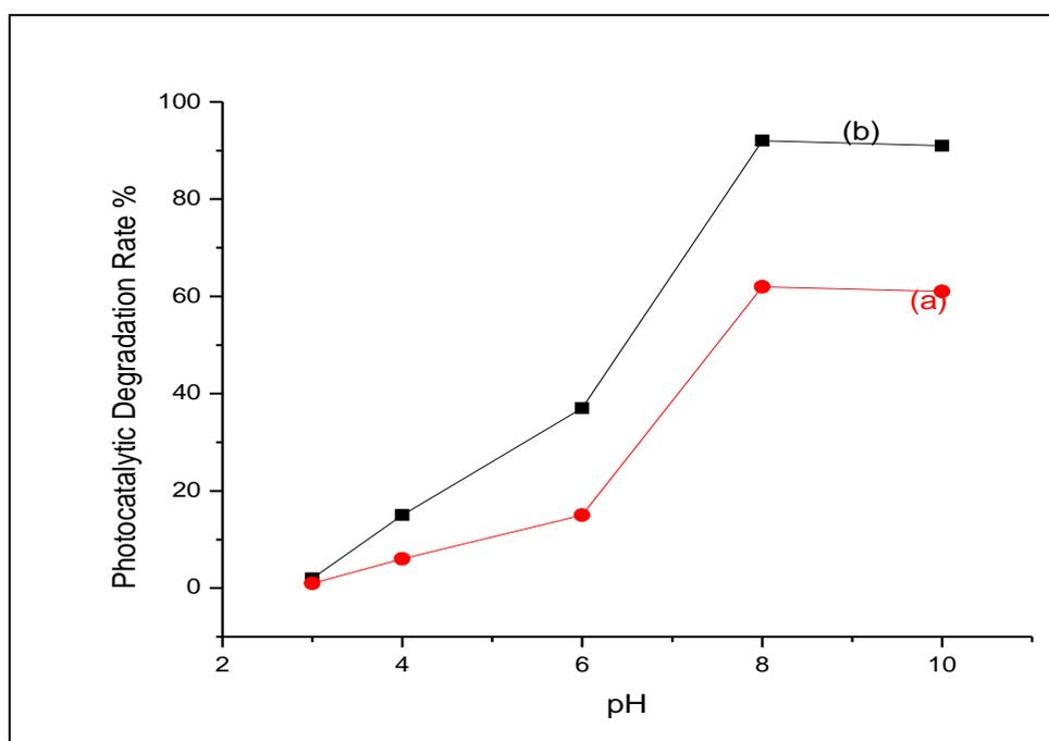
Fig. 3. Effect of pH on the photocatalytic efficiency of MB on (a)  $\alpha$ -ZrP, and (b) Ag-ZrP.  $V = 200$  ml,  $m_{\text{cat}} = 100$  mg,  $t = 2$  h,  $[\text{MB}] = 100$  ppm.
