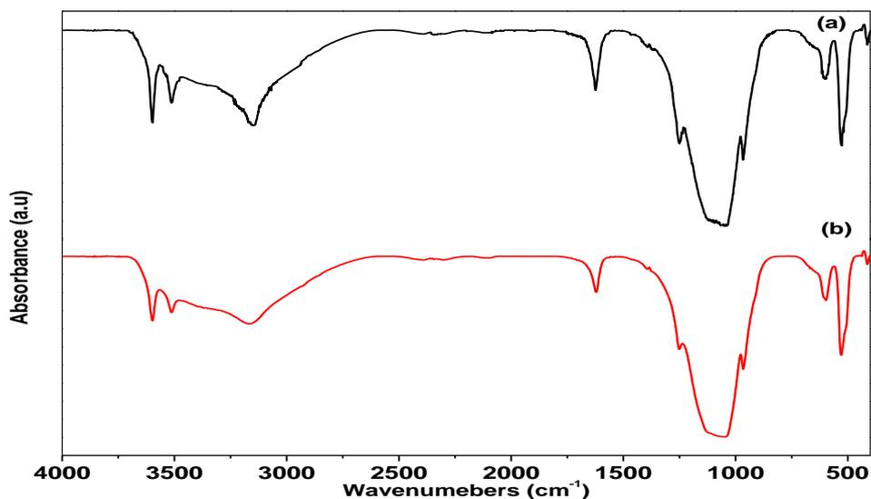
Fig 2. Infrared spectra of (a)  $\alpha$ -ZrP, and (b) Ag-ZrP
