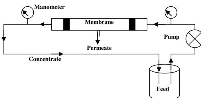
**Fig. 3.** Microfiltration pilot plant scheme.
