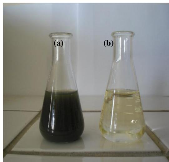
Fig. 11. Effluent before (a) and after (b) treatment using cordierite/ZrO<sub>2</sub> microfiltration membrane.
