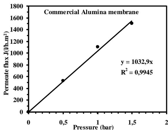
Fig. 5. Variation of water flux as a function of working pressure.
