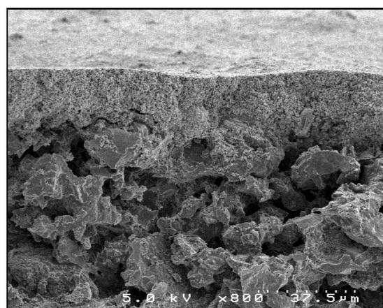
Fig. 2. SEM micrograph of Cordierite/ $\text{ZrO}_2$  membrane (Cross section view).
