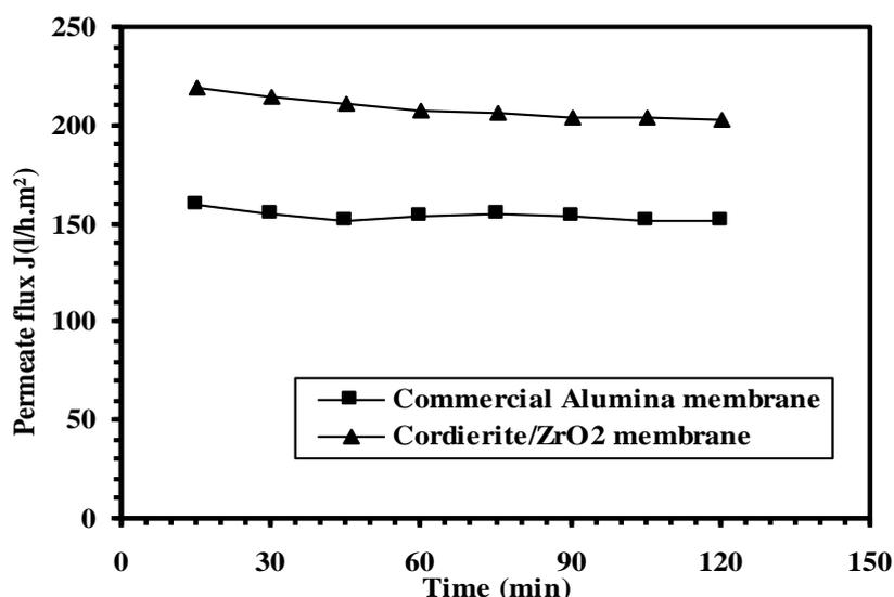
**Fig. 6.** Permeate flux of effluent as a function of operating time.
