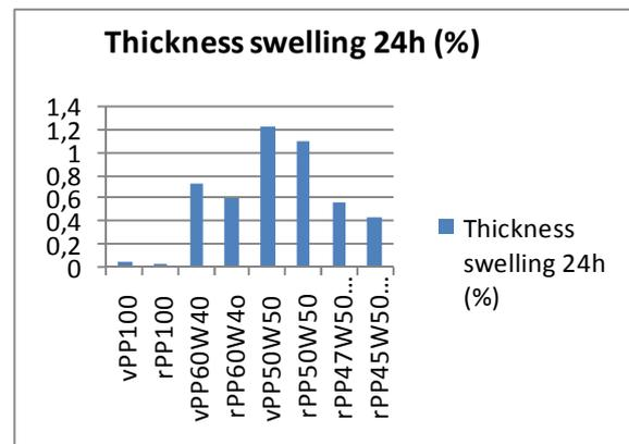
**Fig. 3.** Thickness swelling properties
