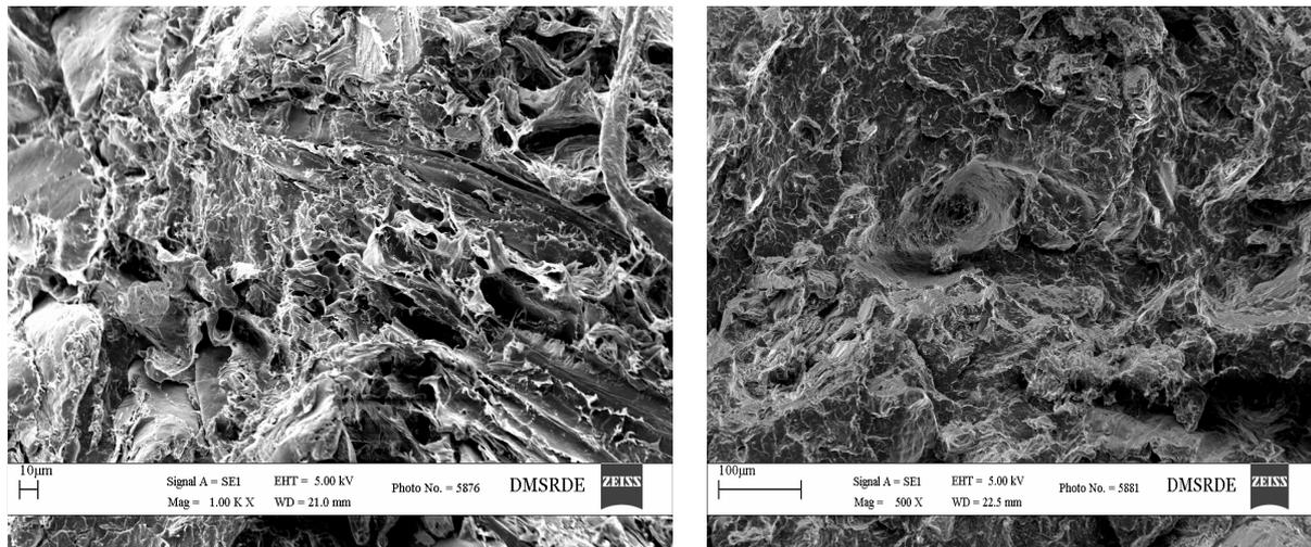
Fig.5. SEM images ( $\times 1000$ ) of fractured surface of (a) rPP47W50CA3, (b) rPP45W50CA5
