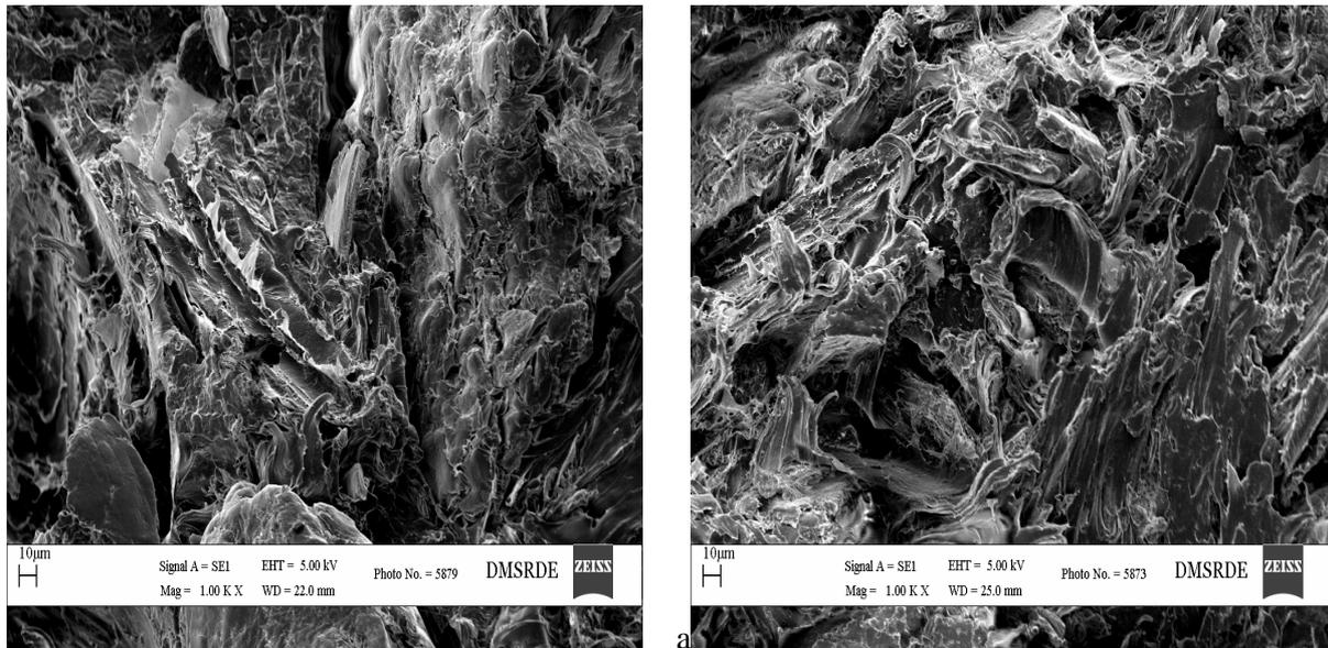
Fig. 4. SEM images ( $\times 1000$ ) of fractured surface of (a) vPP50W50, (b) rPP50W50
