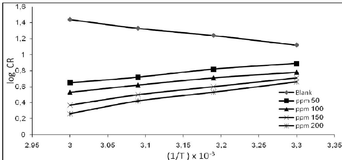
**Fig.6.** Arrhenius plot for C- Steel in 1M HCl solution in the absence and presence of different concentrations of the inhibitor PS.
