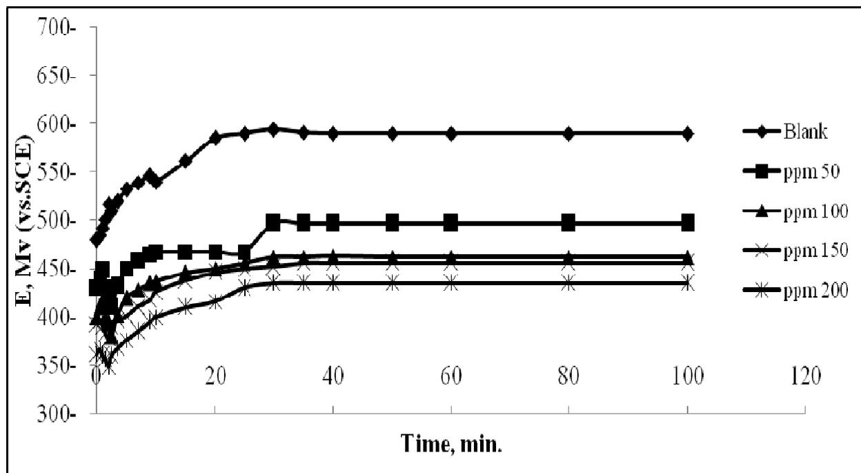
**Fig.2.** Potential–time curves for carbon steel immersed in 1M HCl solution in the absence and presence of different concentrations of (PS).
