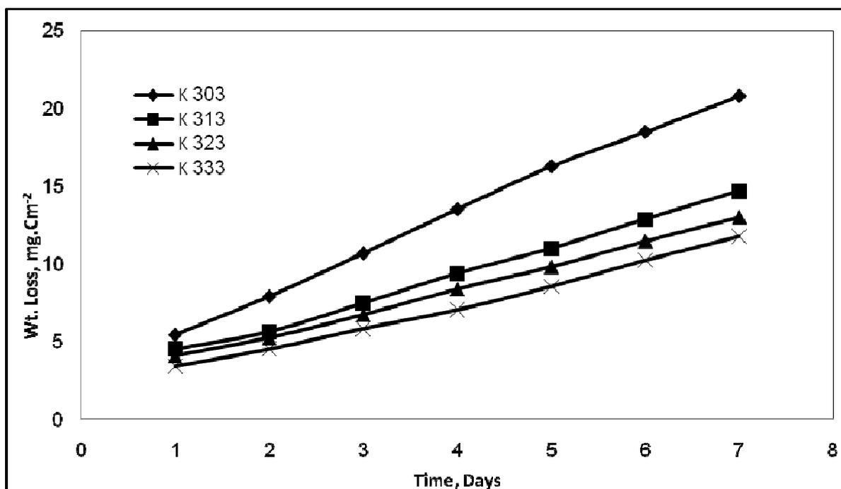
**Fig. 4.** Weight loss-time curves of C-steel alloy in 1 M HCl in the presence of 200 ppm of inhibitor PS at different temperatures
