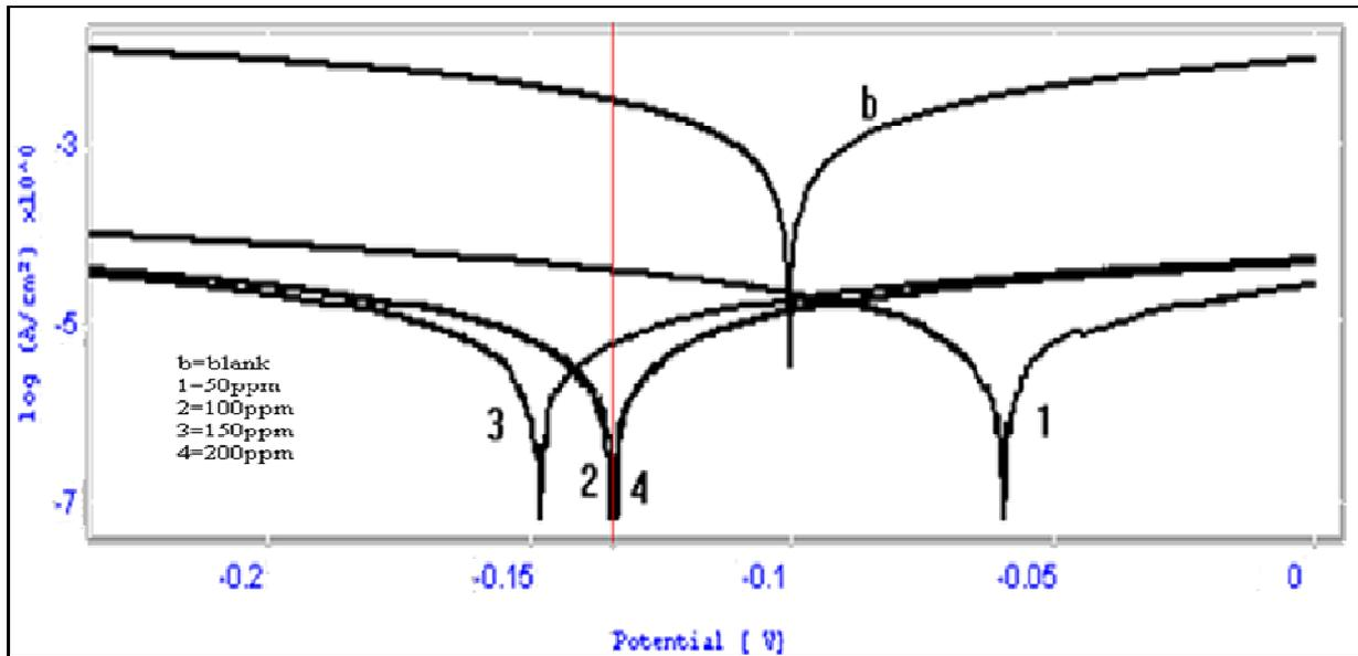
**Fig.3.** Potentiodynamic polarization curves of C-steel in 1 M HCl in absence and presence of different concentrations of inhibitor **PS** at 303 K,
