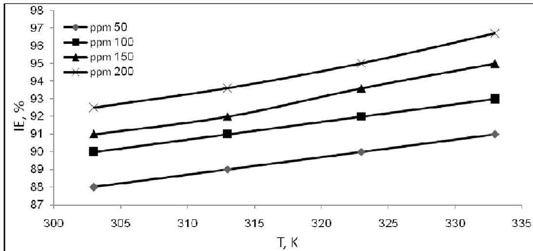
**Fig.5.** Effect of temperature on IE for C- Steel in 1M HCl in the presence of different concentrations of the inhibitor PS.
