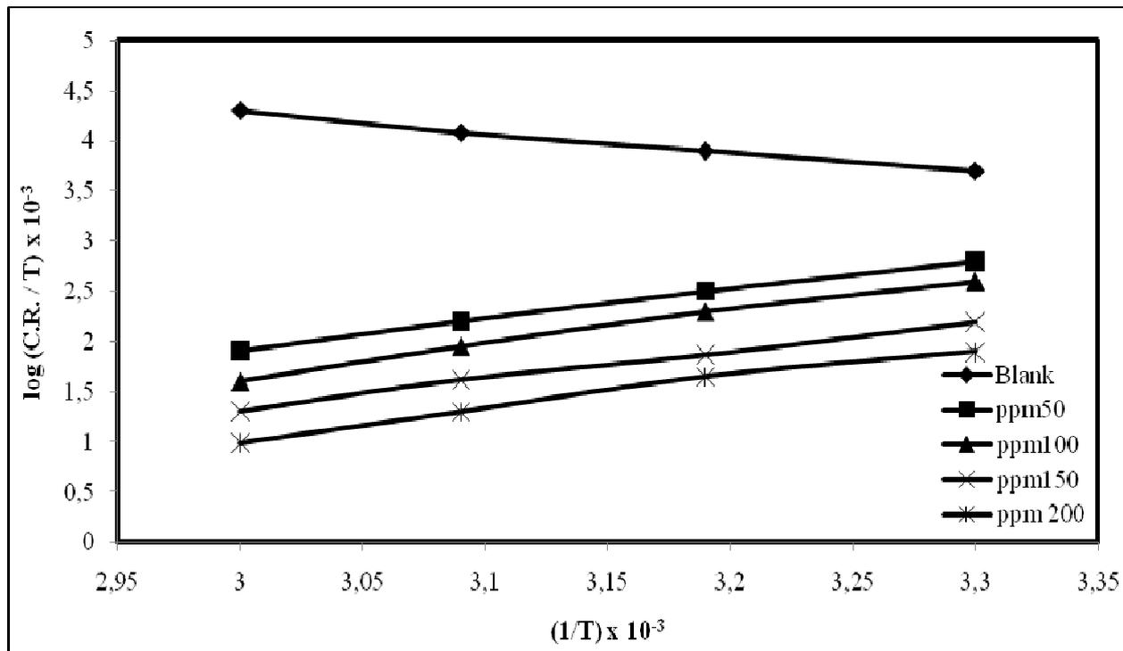
Fig.7. Transition state plot for C-Steel in 1M HCl solution in the absence and presence of different concentrations of the inhibitor PS.
