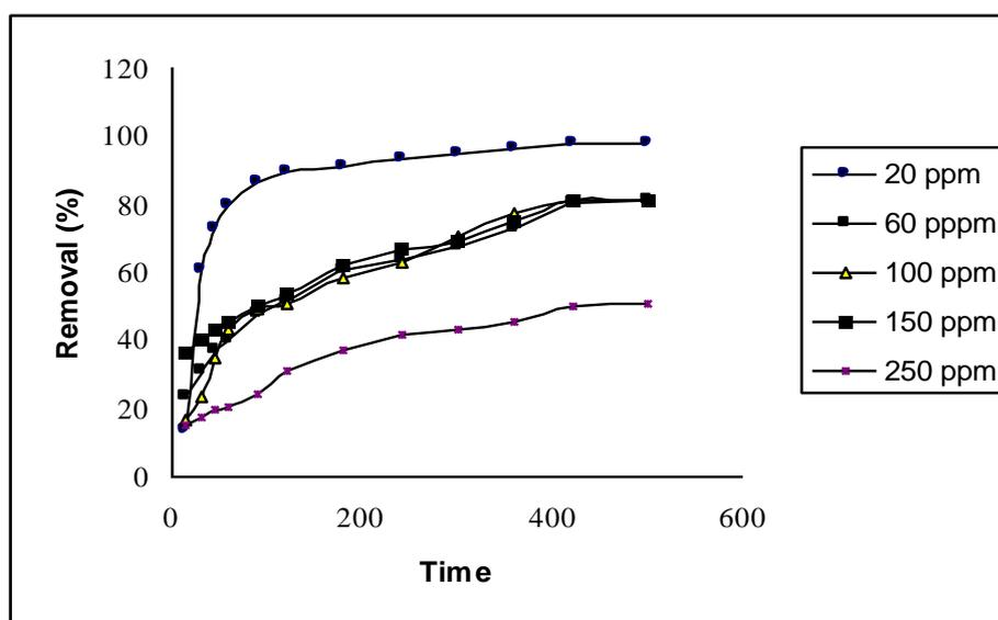
**Figure 1:** Effect of contact time on the removal of RBY dye .Conditions: 4g/L CGT , pH=7 , 50 mL of RBY solution, temperature 25 °C , Agitation speed 180 rpm.
