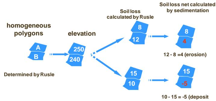
Figure 4: Principle model of deposition: Sedimentation (El Garouani A. 2007)
