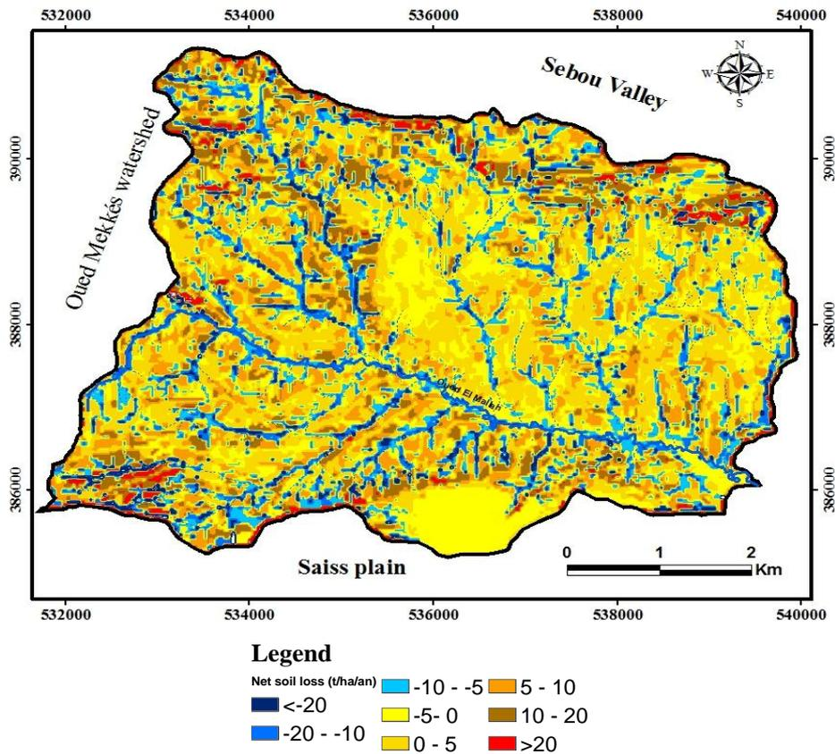
Figure 5: Map of net soil loss determined by the sedimentation model.
