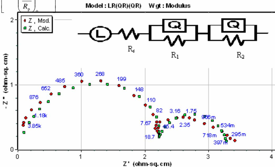
**Figure 3.** The equivalent circuit model used to fit the EIS experimental data of the composite (in the presence of 25 ppm MAMT).
