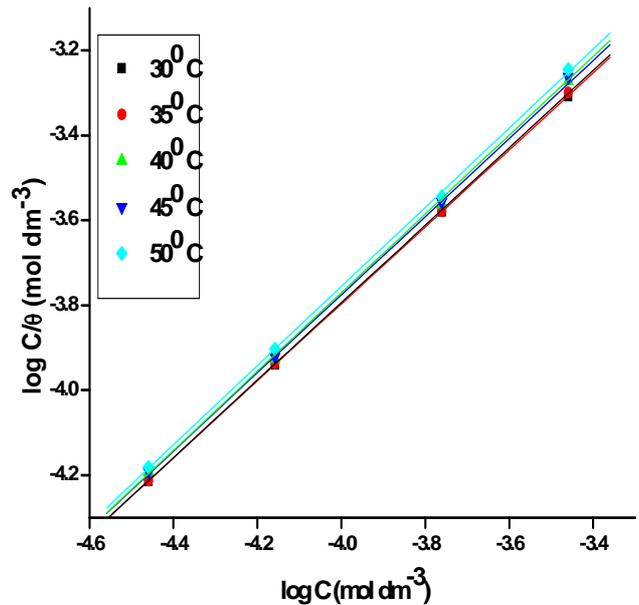
**Figure 6.** Langmuir adsorption isotherms for the adsorption of MAMT on the composite.
