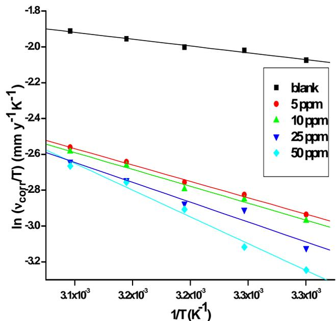
**Figure 5.**  $\ln(v_{\text{corr}}/T)$  vs.  $1/T$  plots for the corrosion of 6061/Al - 15 (vol-%) SiC<sub>(p)</sub> composite in 0.5 M NaOH in the presence of different concentrations of MAMT.
