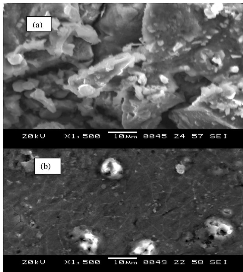
**Figure 8.** SEM images of the surfaces of 6061/Al - 15 (vol-%) SiC<sub>(p)</sub> after immersion for 1 h in 0.5 M NaOH solution at 30 °C (a) in the absence of MAMT (b) in the presence of 50 ppm MAMT.
