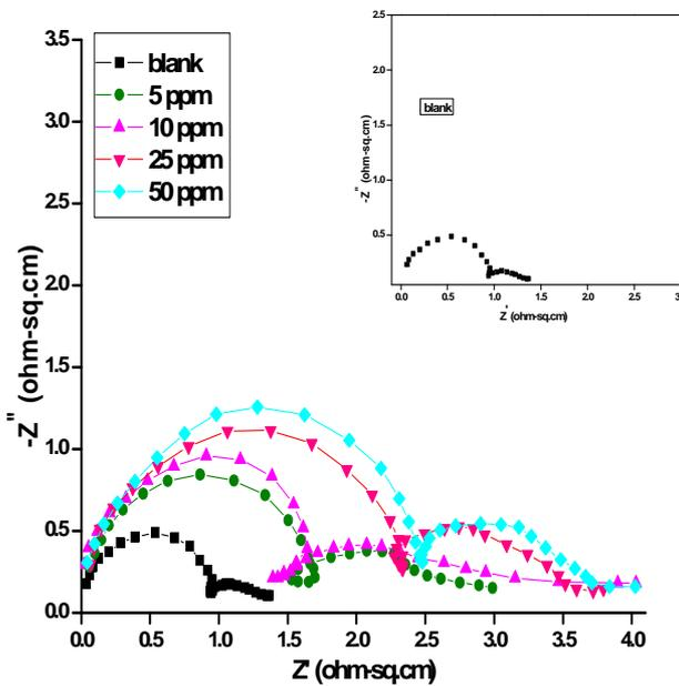
**Figure 2.** Nyquist plots for the corrosion of 6061/Al - 15 (vol-%) SiC<sub>(p)</sub> composite in 0.5 M NaOH at 30 °C in the presence of different concentrations of MAMT.
