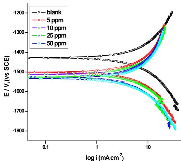
**Figure 1.** Tafel polarization curves for the corrosion of 6061/Al - 15 (vol-%) SiC<sub>(p)</sub> composite in 0.5 M NaOH at 30 °C in the presence of different concentrations of MAMT.
