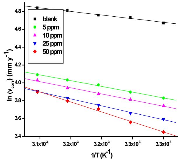
**Figure 4.** Arrhenius plots for the corrosion of 6061/Al-15 (vol-%) SiC<sub>(p)</sub> composite in 0.5 M NaOH in the presence of different concentrations of MAMT.
