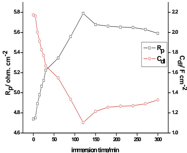
**Figure 7.** The dependence of  $R_p$  and  $C_{dl}$  on the immersion time for the corrosion 6061/Al - 15 (vol-%) SiC<sub>(p)</sub> composite in 0.5 M NaOH in the presence of 50 ppm MAMT at 30 °C.
