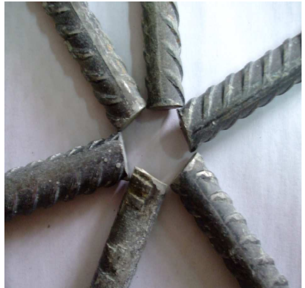
Figure 1.2 Steel embedded in concrete with 3% calcium stearate.
