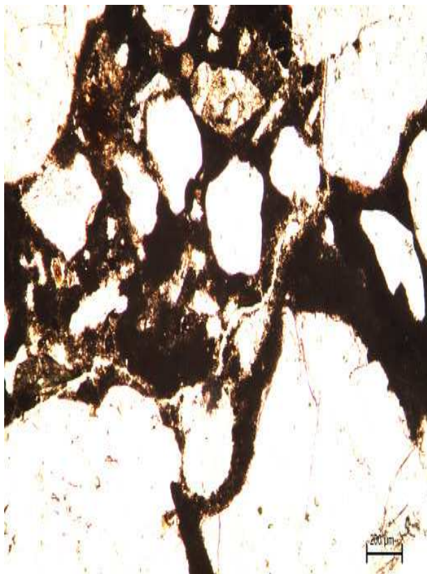
Figure 2.2 Photomicrograph exhibiting that microcracks running along the periphery of coarse aggregate and also within the groundmass of the concrete without calcium stearate.
