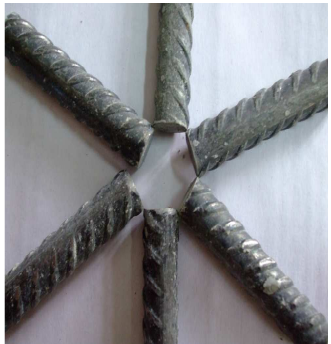
Figure 1.3 Steel embedded in concrete with 5% calcium stearate.
