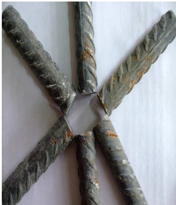
Figure 1.1 corroded bar in control sample.
