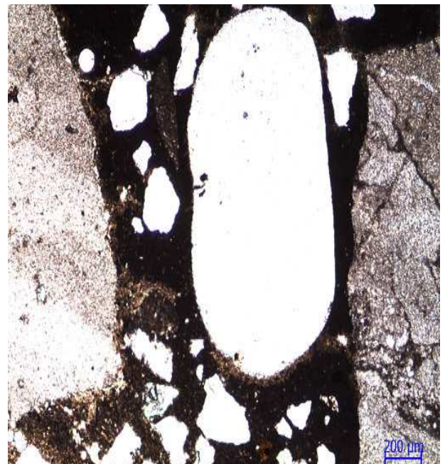
Figure 2.3 Photomicrograph showing the presence of large to small sized voids within the concrete without calcium stearate. Also notice carbonation along the periphery of the large void.
