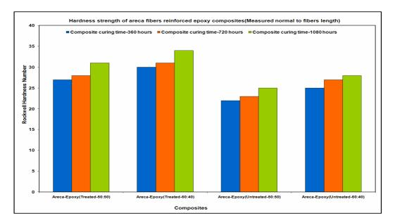
Figure 3. Shows the hardness strength of composites (Measured normal to fiber length)
