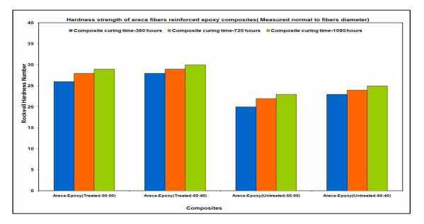
Figure 4. Shows the hardness strength of composites (Measured normal to fiber diameter)
