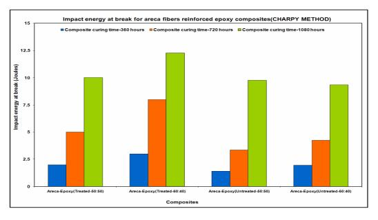
Figure 1. Shows impact energy of composites in Charpy impact test
