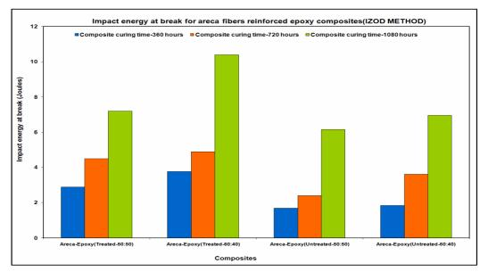
Figure 2. Shows impact energy of composites in Izod impact test
