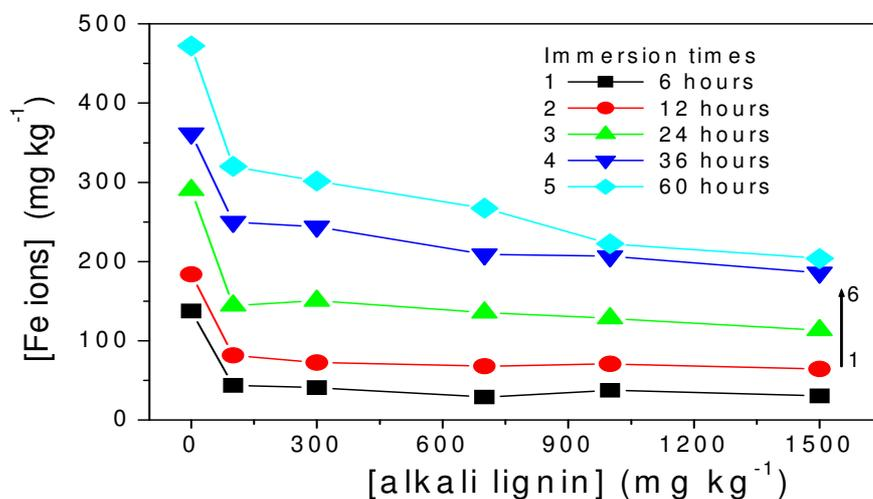
**Figure 8** The variation of Fe ions concentrations in the corrosive solution resulted from stainless steel corrosion in the absence and presence of different concentrations of alkali lignin under different immersion times.
