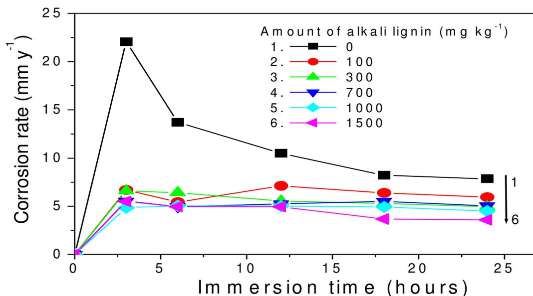
**Figure 2** The corrosion rates of mild steel alloy in 1.0 M HCl in absence and presence of different concentrations of alkali lignin.
