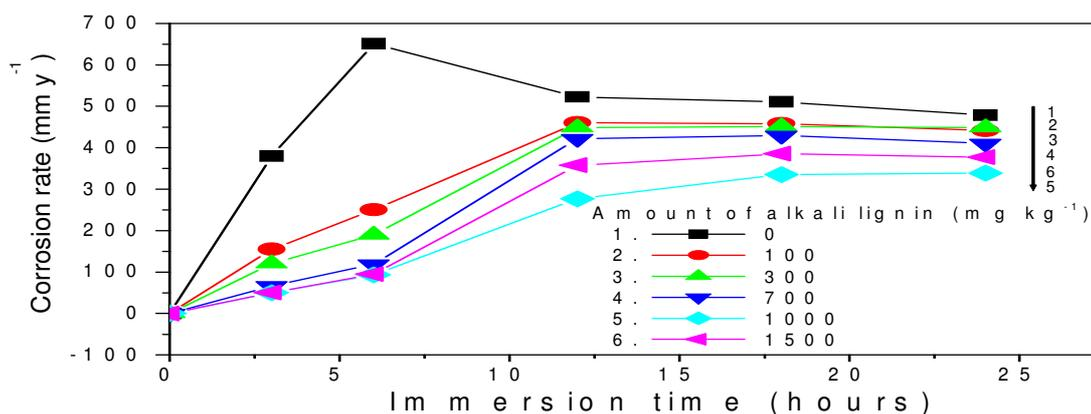
**Figure 3** The corrosion rates of aluminum zinc alloy in 1.0 M HCl in absence and presence of different concentrations of alkali lignin.
