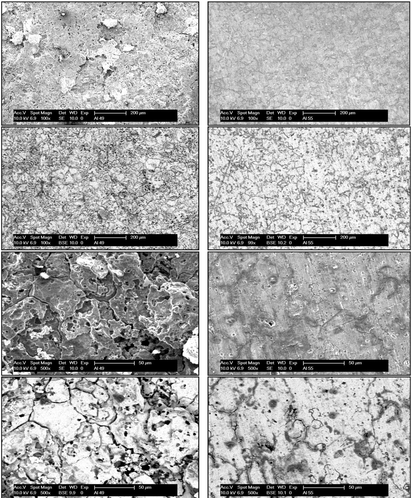
**Figure 10** The SEM images of the corroded surface of aluminum zinc alloy coupons in 0.10 M HCl solutions in the absence (left side) and presence of alkali lignin (right side).
