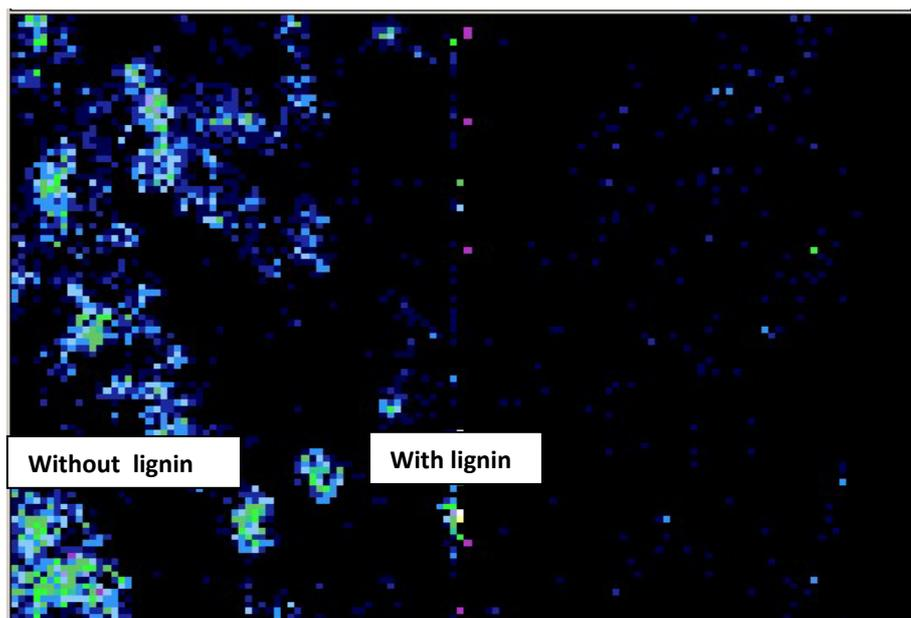
**Figure 11** The mapping images of two different corroded areas on the mild steel coupons immersed in a solution of 1.0 M HCl in the absence and presence of alkali lignin and the distribution images of Cl atoms in the two areas, the hell regions indicate more concentrations of Cl atoms.
