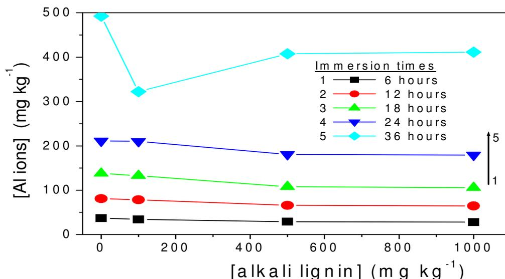
**Figure 7** The variation of Al ions concentrations in the corrosive solution (0.40 M HCl) resulted from Al alloy corrosion in absence and presence of different concentrations of alkali lignin under different immersion times.
