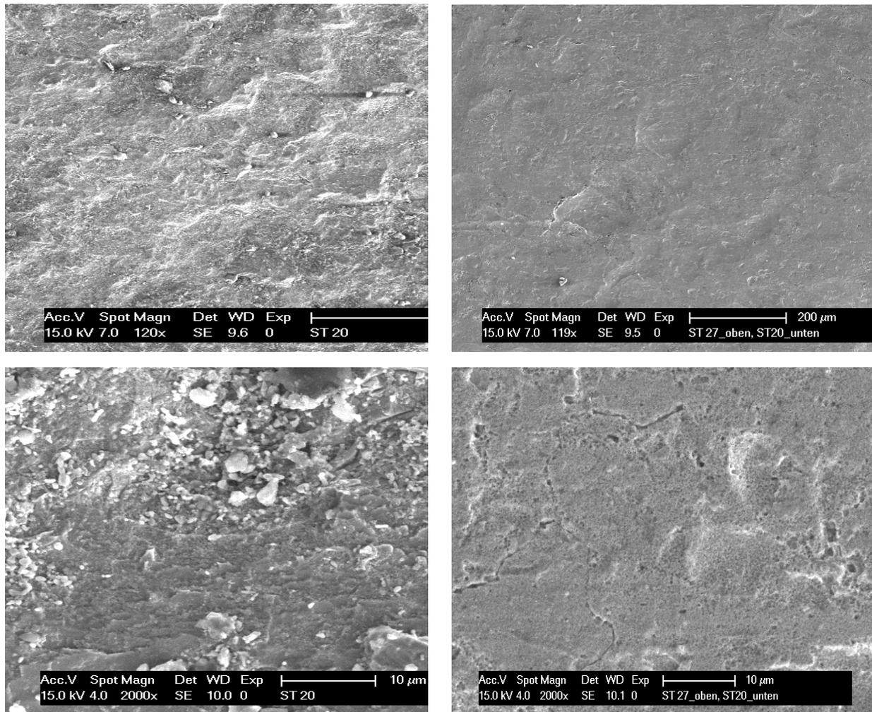
**Figure 9** The SEM images of the corroded surface of mild steel coupons in 0.10 M HCl solution in the absence (left side) and presence of alkali lignin (right side).
