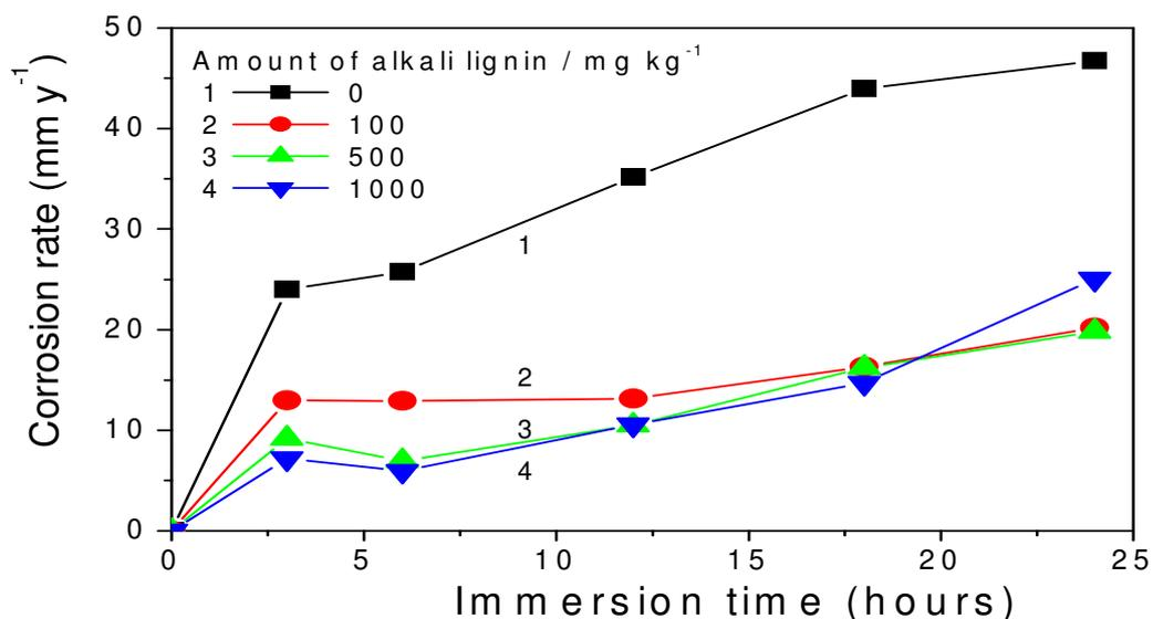
**Figure 5** The corrosion rates of aluminum zinc alloy in 0.40 M HCl in absence and presence of different concentrations of alkali lignin.
