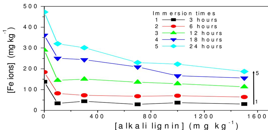
**Figure 6** The variation of Fe ions concentrations in the corrosive solution (1.0 M HCl) resulted from mild steel corrosion in absence and presence of different concentrations of alkali lignin under different immersion times.
