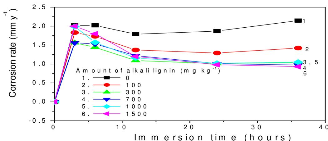
**Figure 4** The corrosion rates of aluminum zinc alloy in 0.10 M HCl in absence and presence of different concentrations of alkali lignin.
