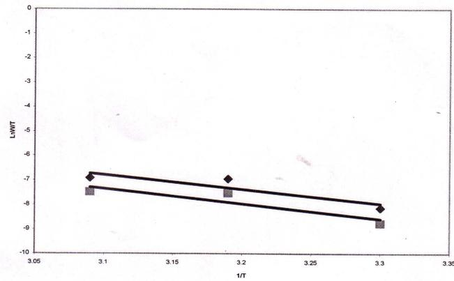
**Fig. 9:** Arrhenius plots of  $\ln w/T$  Vs  $1/T$  at pH 4  $\blacklozenge$  without inhibitor  $\blacksquare$  with 100 ppm inhibitor
