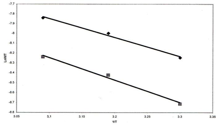
**Fig. 8:** Arrhenius plots of  $\ln w/T$  Vs  $1/T$  at pH 6  $\blacklozenge$  without inhibitor  $\blacksquare$  with 100ppm inhibitor
