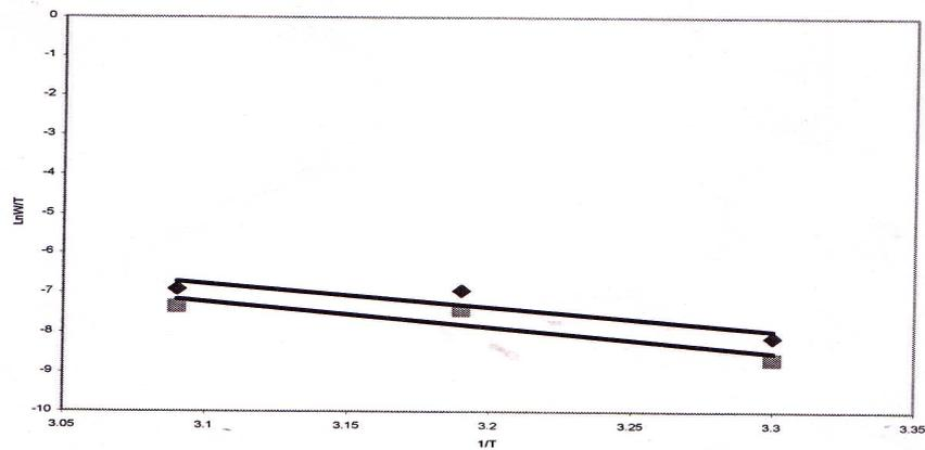
**Fig. 11:** Arrhenius plots of  $\ln w/T$  Vs  $1/T$  at pH 4  $\blacklozenge$  without inhibitor  $\blacksquare$  with 50 ppm inhibitor
