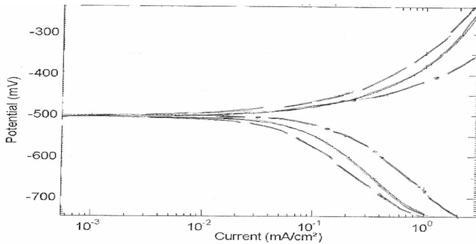
**Fig. 1.** Polarization curves for mild steel at pH 6 at different temperature (—●—) 30 °C, (—) 40 °C, (---) 50 °C
