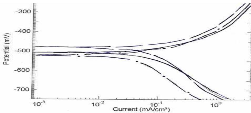
**Fig. 4.** Polarization curves for mild steel at pH 4 containing 50 ppm amine melamine formaldehyde resin at different temperature (---) 30 °C, (—)40 °C, (-●-) 50 °C
