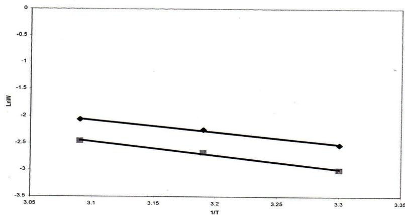
**Fig. 6:** Arrhenius plots of  $\ln w$  Vs  $1/T$  at pH 6 ♦ without inhibitor ■ with 100ppm inhibitor
