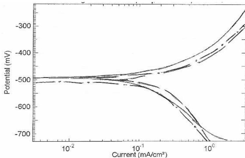
**Fig. 2.** Polarization curves for mild steel at pH 4 at different temperature (—) 30 °C, (---) 40 °C, (—●—) 50 °C
