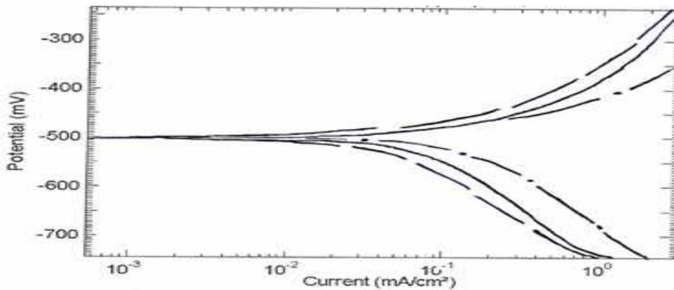
**Fig. 5.** Polarization curves for mild steel at pH 4 containing 100 ppm amine melamine formaldehyde resin at different temperature (---) 30 °C, (—)40 °C, (-●-) 50 °C
