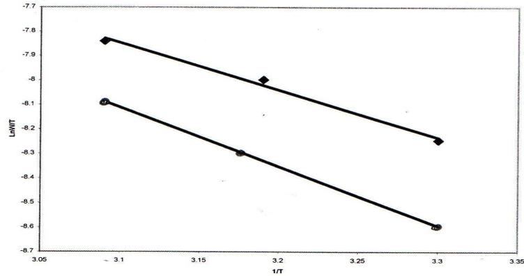
**Fig. 10:** Arrhenius plots of  $\ln w/T$  Vs  $1/T$  at pH 6  $\blacklozenge$  without inhibitor  $\blacksquare$  with 50 ppm inhibitor
