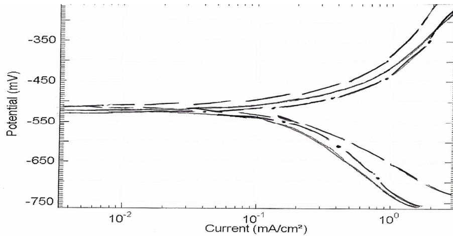
**Fig. 3.** Polarization curves for mild steel at pH 6 containing 50 ppm amine melamine formaldehyde resin at different temperature (---) 30 °C, (—)40 °C, (-●-) 50 °C
