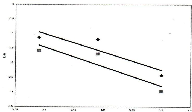
**Fig. 7:** Arrhenius plots of  $\ln w$  Vs  $1/T$  at pH 6 ♦ without inhibitor ■ with 50 ppm inhibitor
