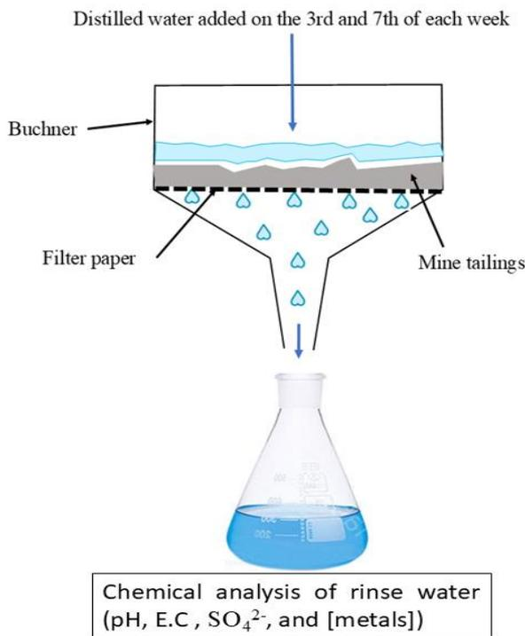
**Figure 1:** Schematic diagram summarizing Mini-Cell Alteration tests (Bussière *et al.*, 2005, adapted from Cruz *et al.*, 2001)
