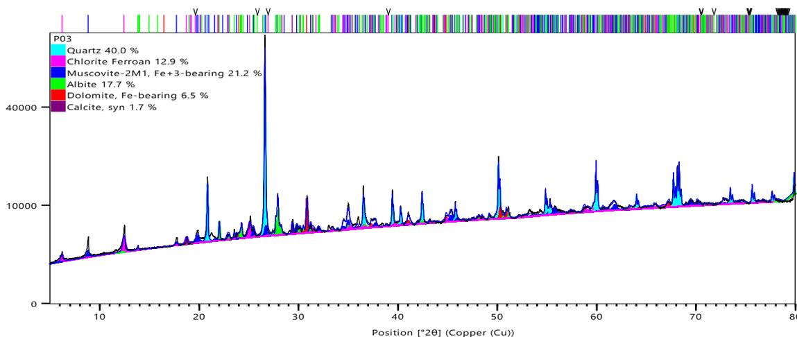
**Figure 2:** XRD spectrum of mine tailings
