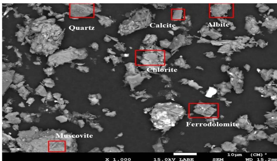
**Figure 3:** Electronic image Various carbonates (calcite, dolomite) and silicates (quartz, muscovite, albite and chlorite) found in Sabodala mine tailings.
