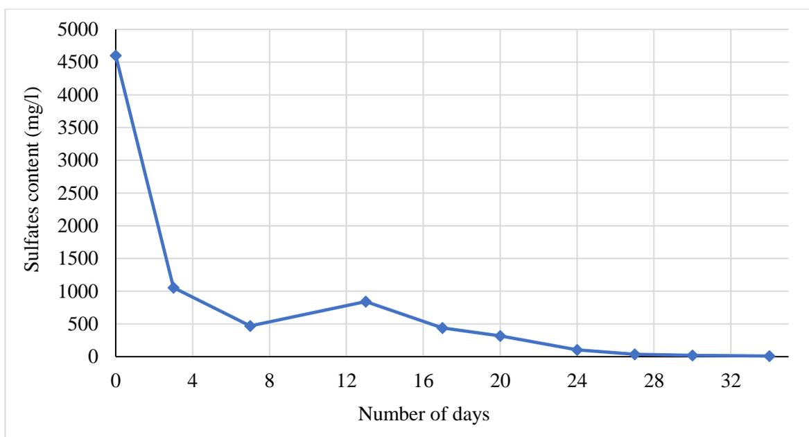
**Figure 6:** Changes in sulfate levels in ACM leachates as a function of time
