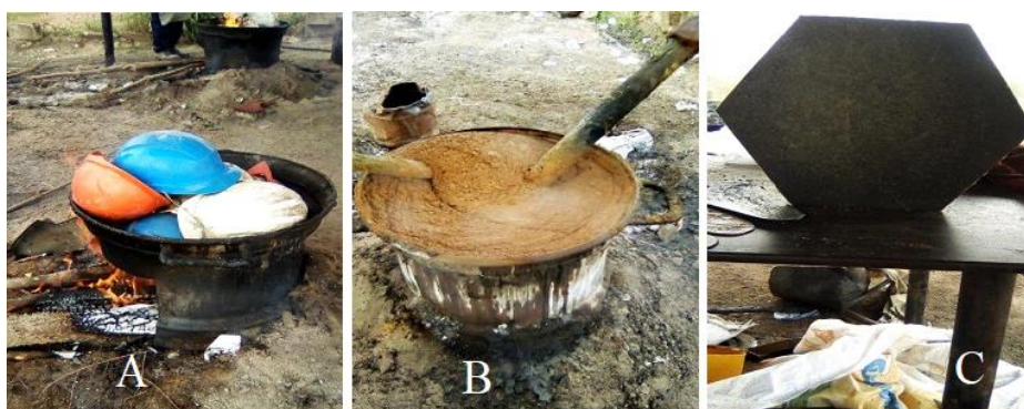
Figure 5. Recycling of plastic waste (A : incineration of plastics ; B : addition of sand; C : finished « pavement » product)
