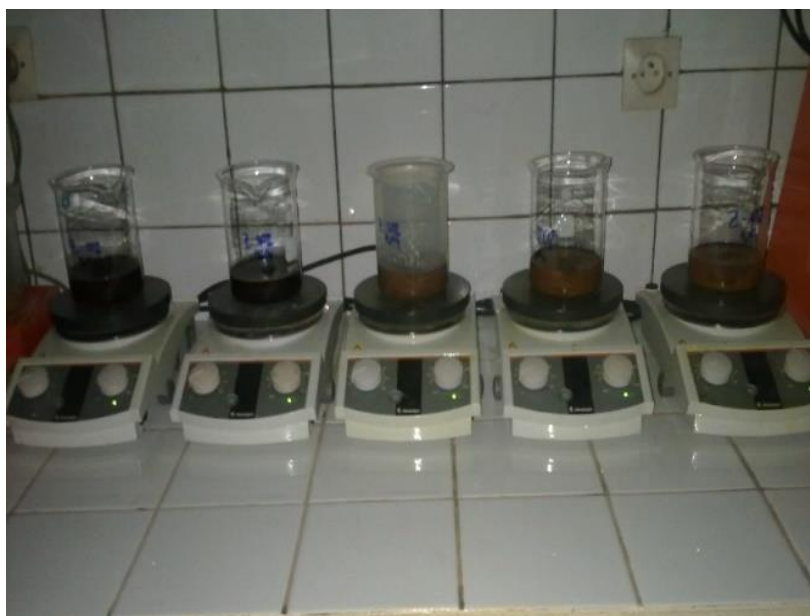
Figure 3. Impregnation on magnetic stirrers
