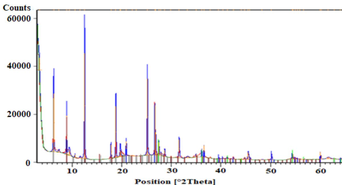
**Figure 5:** X-ray diffractogram of clay-TiO<sub>2</sub>
