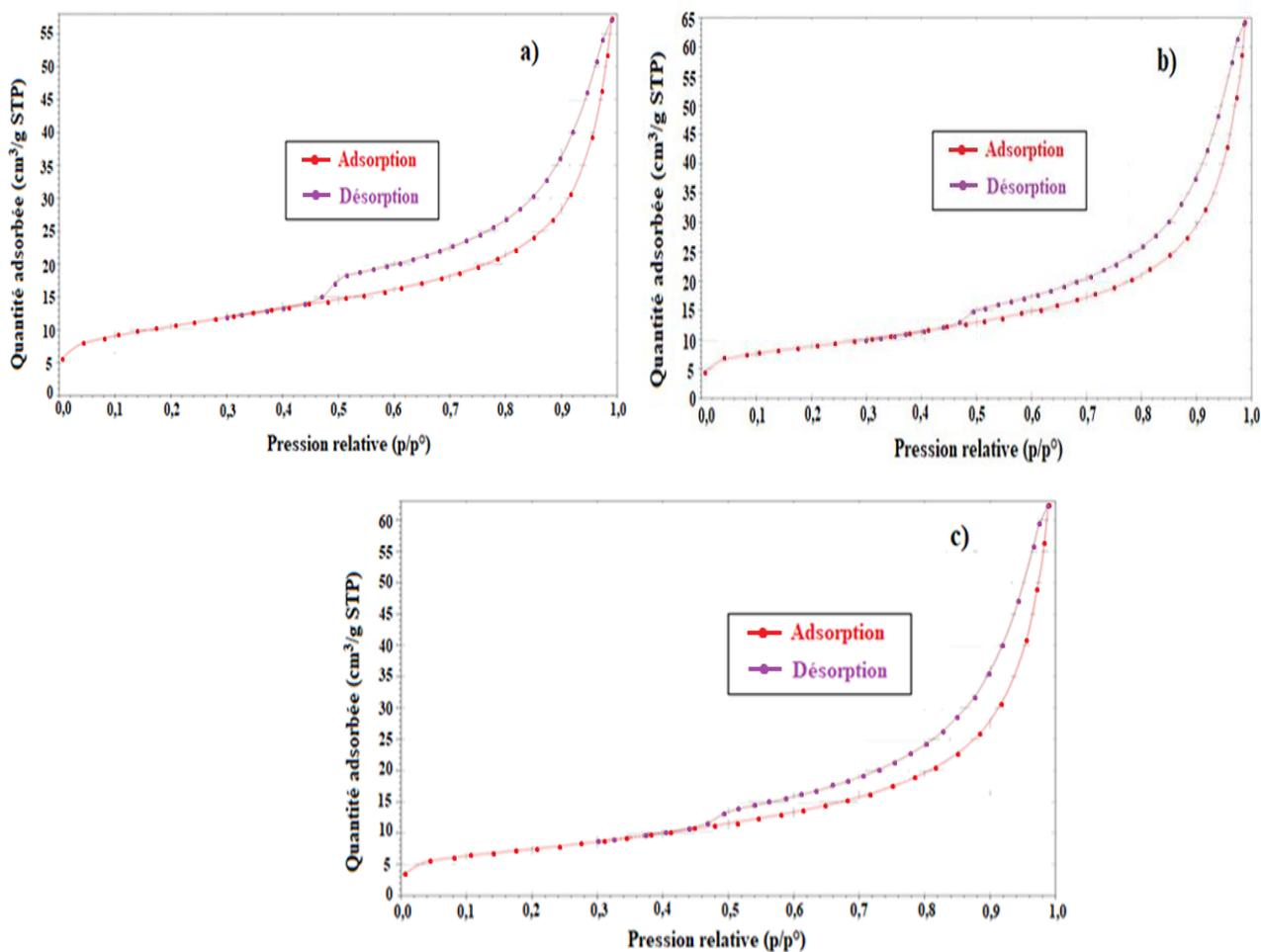
**Figure 8:** Adsorption and desorption isotherms for nitrogen at 77 K on clay, (a): raw clay; (b): calcined clay; (c): clay-TiO<sub>2</sub>
