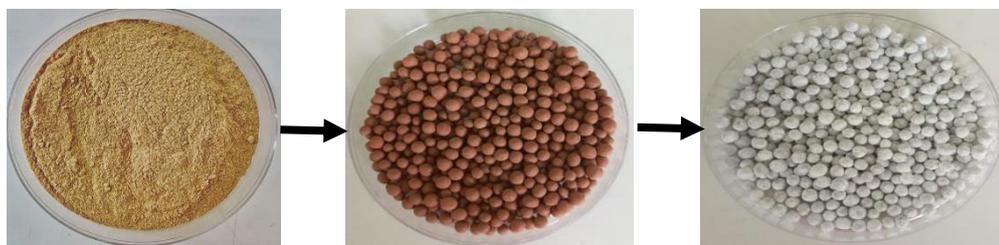
**Figure 2:** Preparation steps of the supported photocatalyst (clay-TiO<sub>2</sub>)
