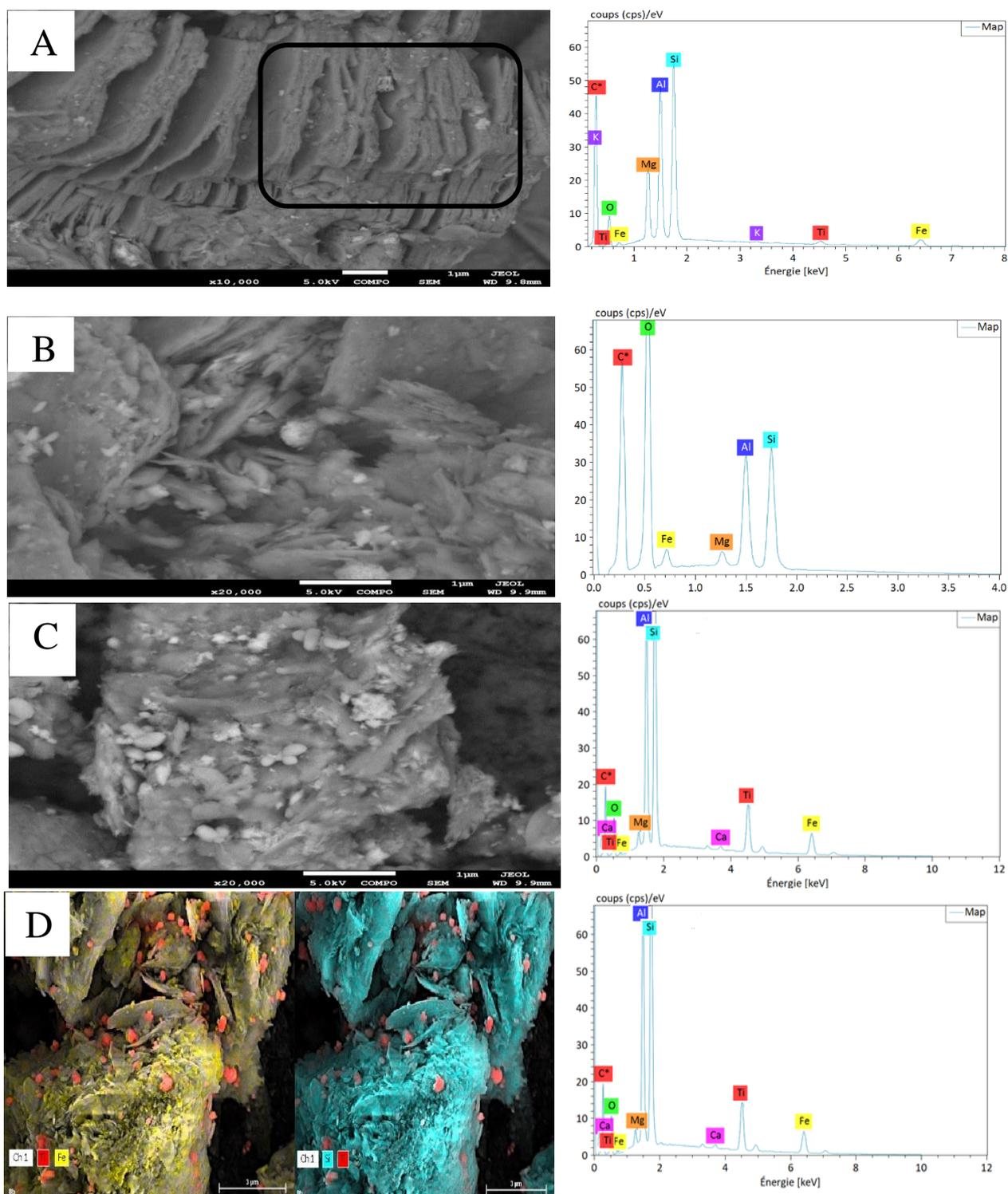
**Figure 7:** SEM micrographs and associated EDS spectra of raw clay (A), calcined clay (B) and clay-TiO<sub>2</sub> (C); Chemical mapping of clay-TiO<sub>2</sub> (D)
