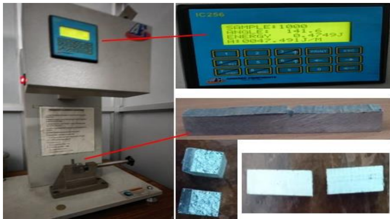
Figure 2. Izod Testing Setup
