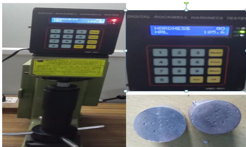
Figure 3. Rockwell Hardness Test Setup
