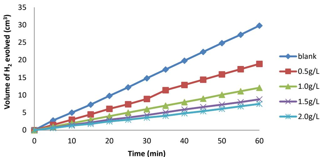
**Figure 3:** Volume – time curve obtained in the absence and presence of various concentrations of *T. occidentalis* stem extract on mild steel in 1 M H<sub>2</sub>SO<sub>4</sub> solution at 30 °C
