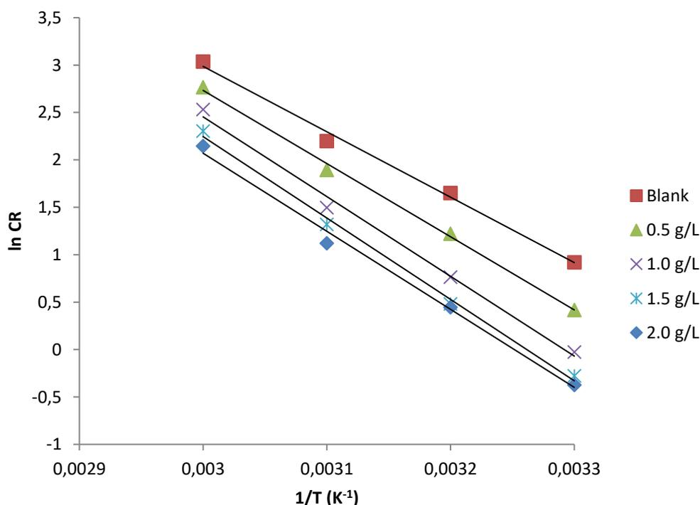
**Figure 4:** Arrhenius plot for mild steel corrosion in 1 M  $H_2SO_4$  in the absence and presence of TOSE
