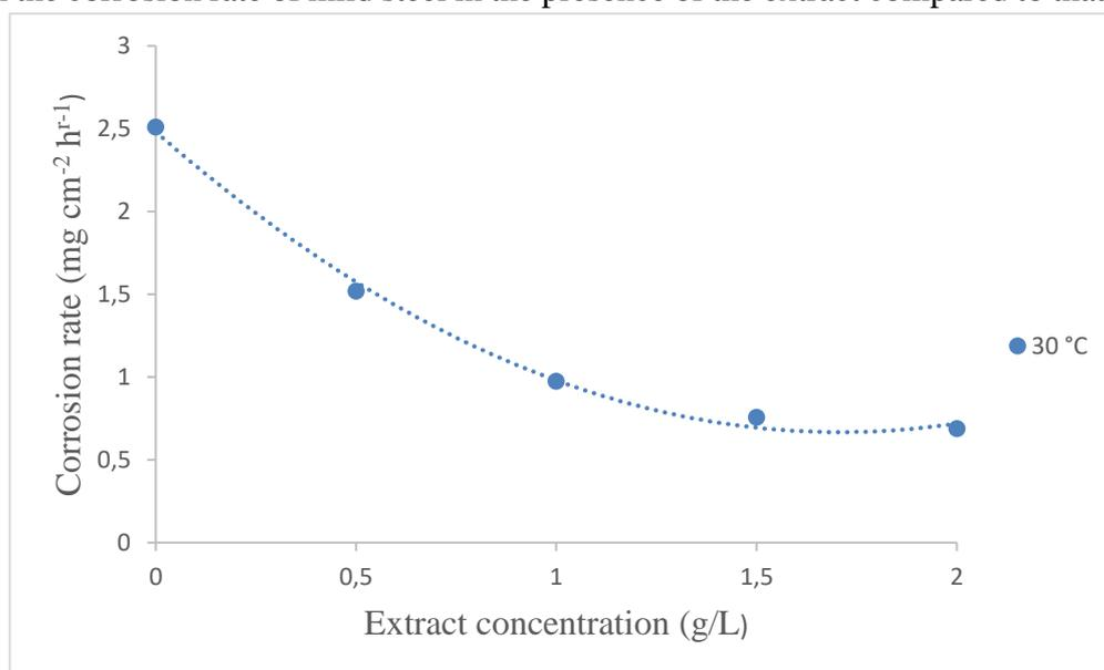
Figure 1: Effect of *T. occidentalis* stem extract concentration on the corrosion rate of mild steel in 1 M  $H_2SO_4$  solution at 30 °C
