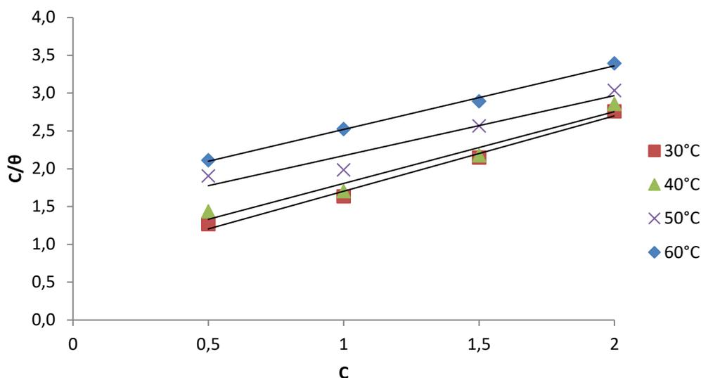
**Figure 6:** Langmuir isotherm for mild steel corrosion in 1 M  $H_2SO_4$  in the absence and presence of TOSE
