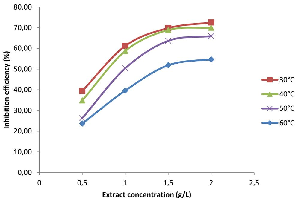
Figure 2: Effect of *T. occidentalis* stem extract (TOSE) concentration on inhibition efficiency of mild steel in 1 M H<sub>2</sub>SO<sub>4</sub> solution
