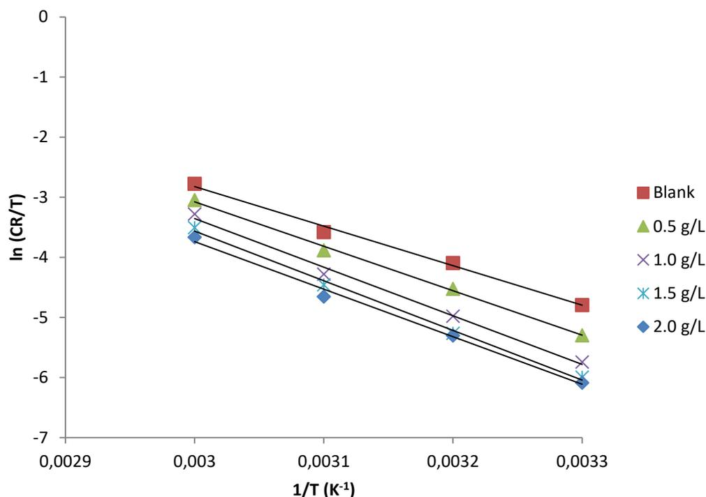
**Figure 5:** Transition State plot for mild steel corrosion in 1 M H<sub>2</sub>SO<sub>4</sub> in the absence and presence of TOSE
