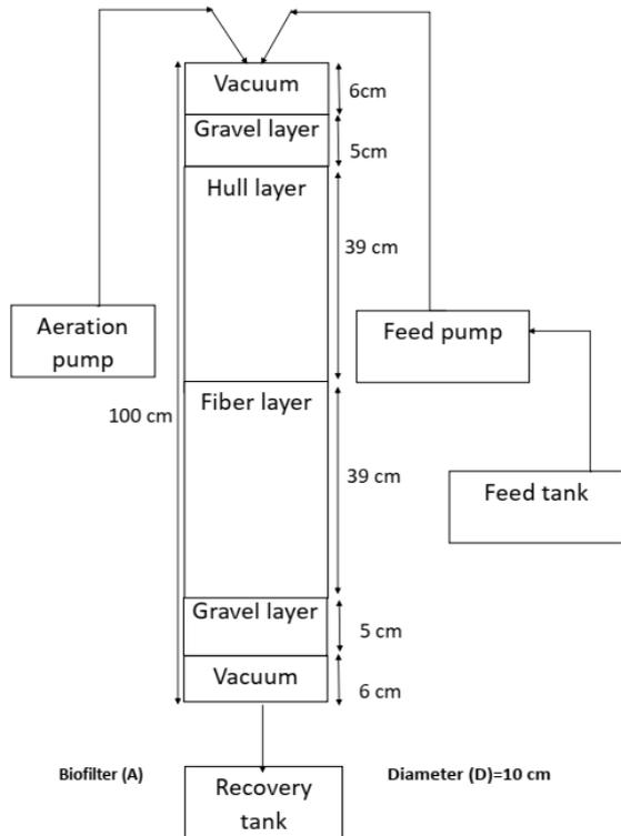
**Figure 8a** : Biofilter A operating diagram
