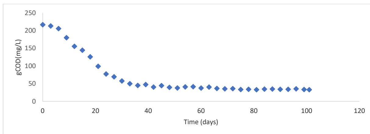
**Figure 11 :** Changes in gross chemical oxygen demand (gCOD) at the pilot plant outlet over time.
