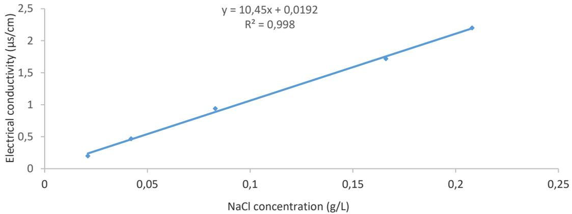
**Figure 9** : Linear regression between electrical conductivity and sodium chloride (NaCl) concentration
