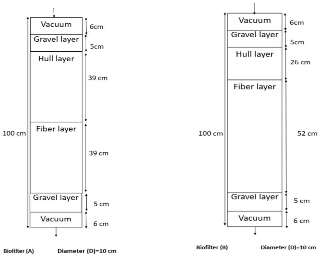
**Figure 5a** : Diagram of the biofilter A
