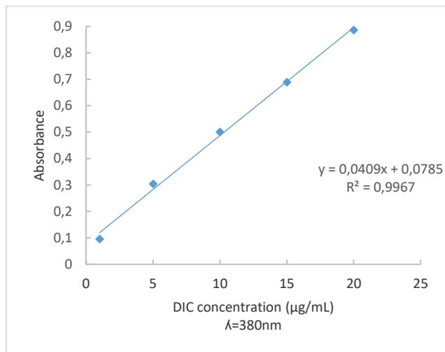
**Figure 12a** : linear regression between absorbance and diclofenac concentration (DIC)
