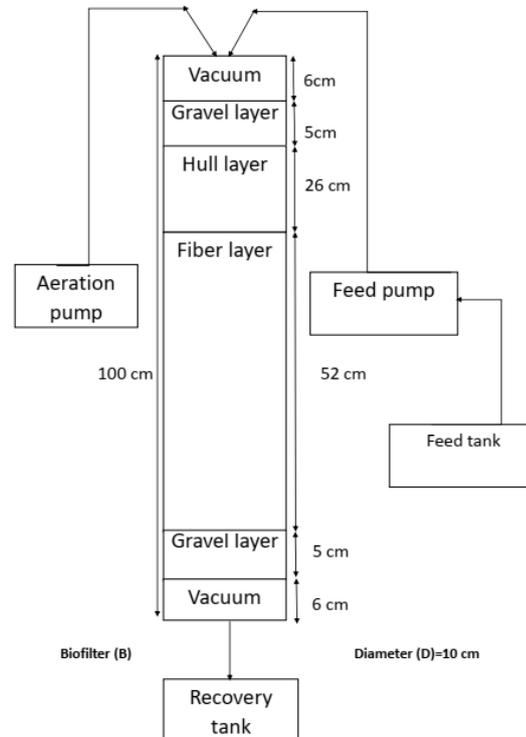
**Figure 8b** : Biofilter B operating diagram
