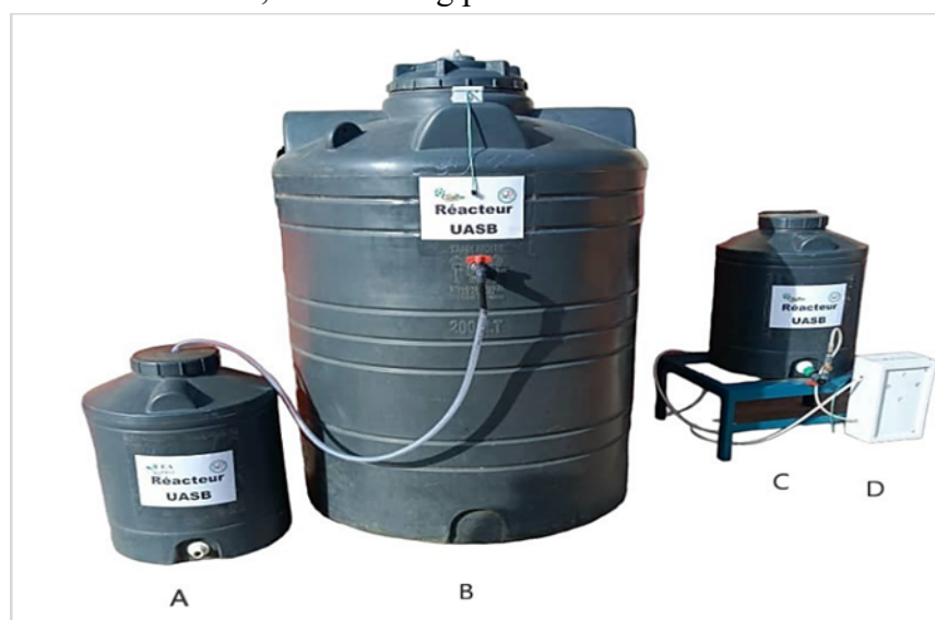
Figure 1. Experimental UASB reactor setup created by CEA-VALOPRO
