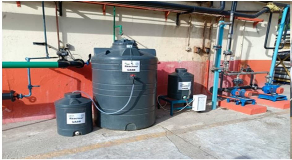
Figure 2. Experimental UASB reactor setup installed at SANIA-cie
