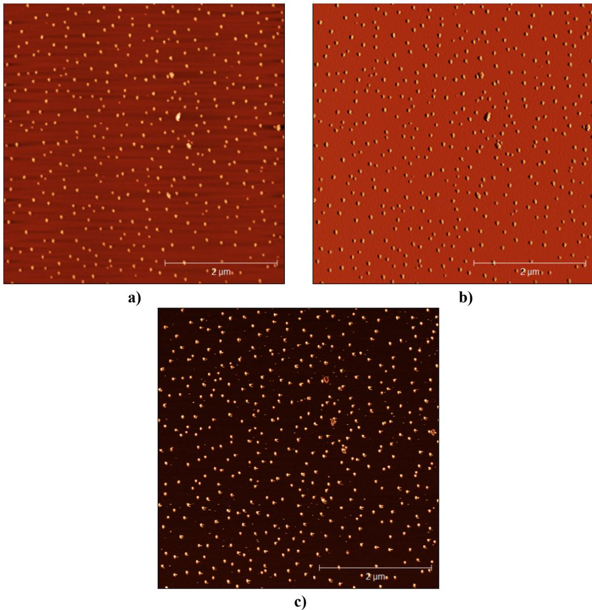
**Figure 6.** AFM image of  $\text{Fe}_3\text{O}_4$  nanoparticles **a)** topography of  $\text{Fe}_3\text{O}_4$  nanoparticles **b)** amplitude of  $\text{Fe}_3\text{O}_4$  nanoparticles **c)** phase of  $\text{Fe}_3\text{O}_4$  nanoparticles
