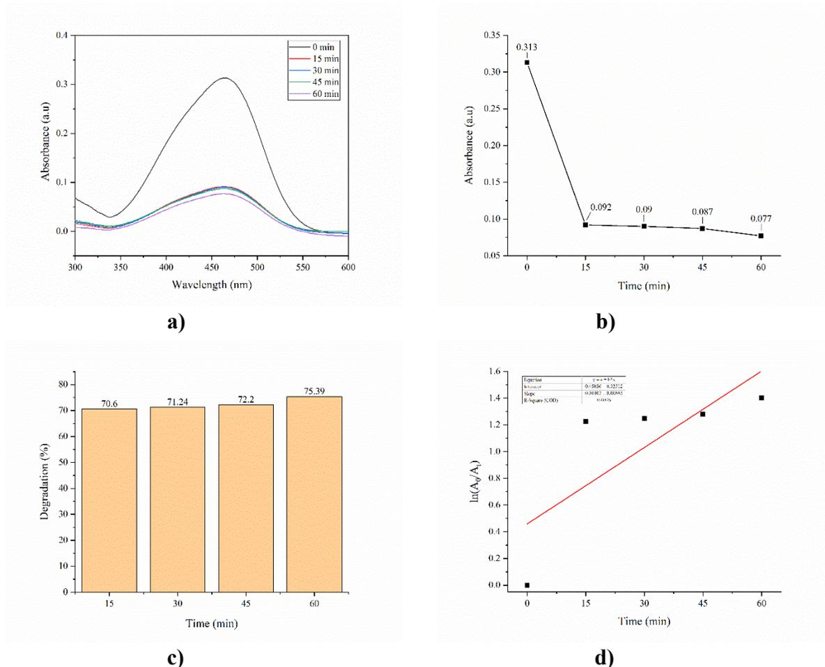
**Figure 9.** a) Absorbance vs wavelength curves of MO at different time intervals b) Absorbance vs time curve of MO c) Degradation of MO by  $\text{Fe}_3\text{O}_4$  nanoparticles at different time intervals d) The kinetic plot of MO
