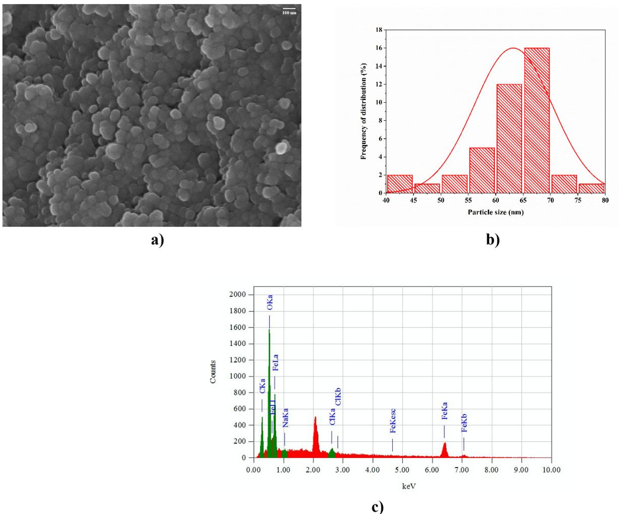
**Figure 4.** a) FESEM image of  $\text{Fe}_3\text{O}_4$  nanoparticles b) Size distribution of  $\text{Fe}_3\text{O}_4$  nanoparticles c) EDAX image of  $\text{Fe}_3\text{O}_4$  nanoparticles
