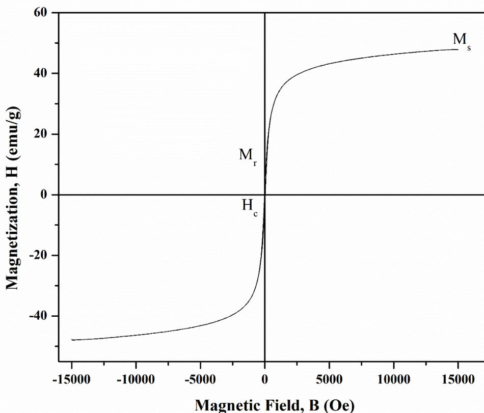
**Figure 7.** B-H (hysteresis) curve of  $Fe_3O_4$  nanoparticles
