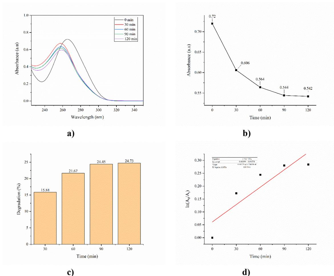
**Figure 10.** **a)** Absorbance vs wavelength curves of SMX at different time intervals **b)** Absorbance vs time curve of SMX **c)** Degradation of SMX by  $\text{Fe}_3\text{O}_4$  nanoparticles at different time intervals **d)** The kinetic plot of SMX
