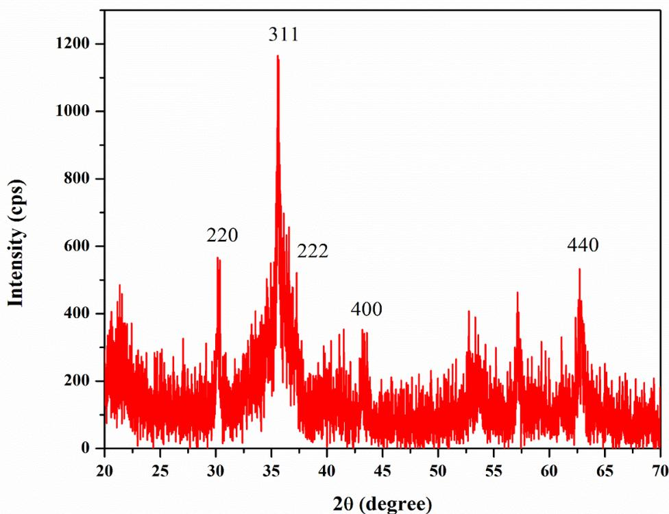
**Figure 2.** XRD pattern of Fe<sub>3</sub>O<sub>4</sub> nanoparticles
