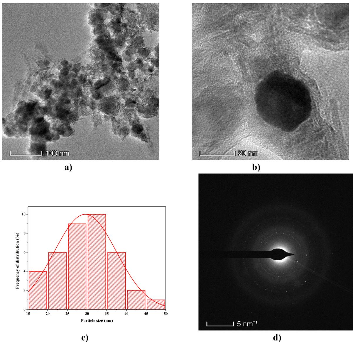
**Figure 5.** a) TEM image of Fe<sub>3</sub>O<sub>4</sub> nanoparticles b) HRTEM image of Fe<sub>3</sub>O<sub>4</sub> nanoparticles c) Size distribution of Fe<sub>3</sub>O<sub>4</sub> nanoparticles d) SAED pattern of Fe<sub>3</sub>O<sub>4</sub> nanoparticles
