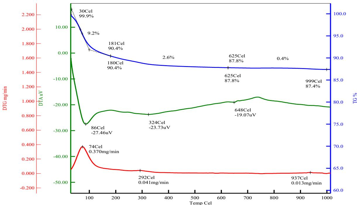
Figure 8. TG-DTA curve of  $\text{Fe}_3\text{O}_4$  nanoparticles
