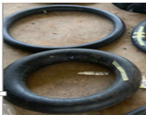
Figure 13: Air chambers containing biogas and samples
