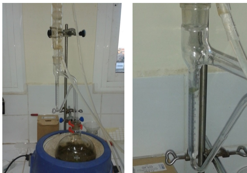
Figure 2. Clevenger device for extracting essential oils.
