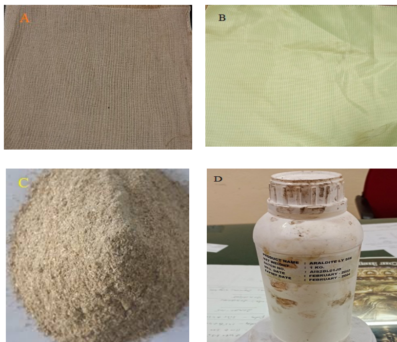
Figure 1. A. fibre ramie B. fibre kevlar C. rice husk and D. epoxy resin
