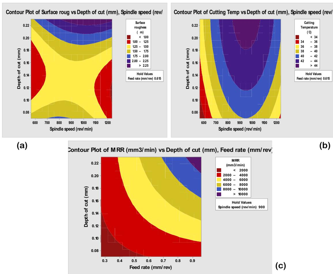
**Figure 6:** Contour plots for responses of MBCF (a) surface roughness (b) cutting temperature (c) MRR
