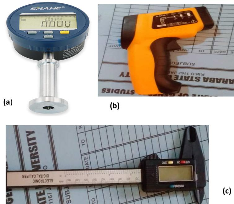
**Figure 3:** Machining materials (a) surface roughness tester (b) infrared pyrometer (c) digital vernier caliper
