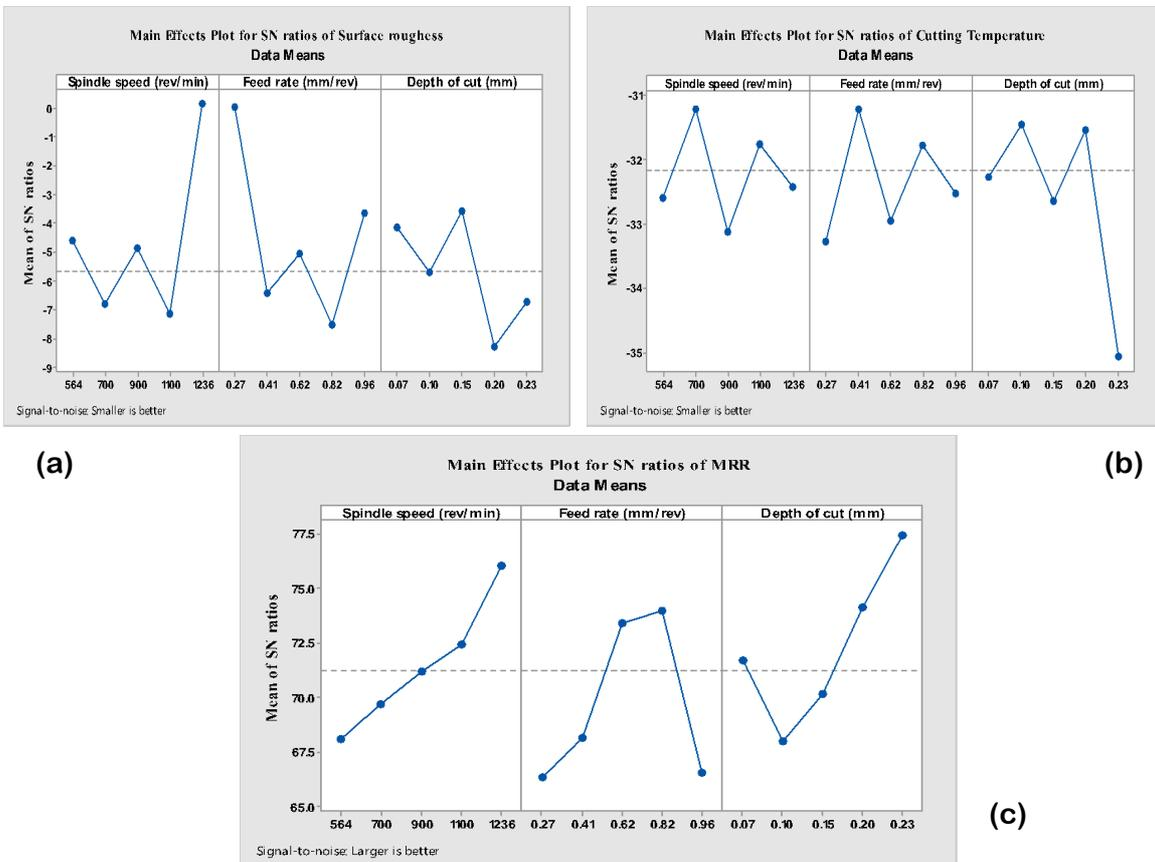
Figure 5: Main effect plots for responses of CBCF (a) surface roughness (b) cutting temperature (c) MRR
