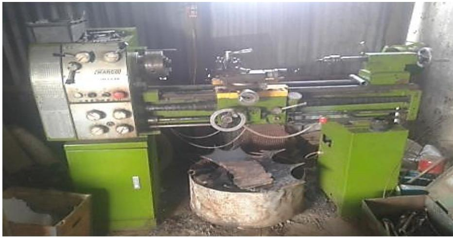
**Figure 2:** Three-jaw chuck lathe machine used for machining
