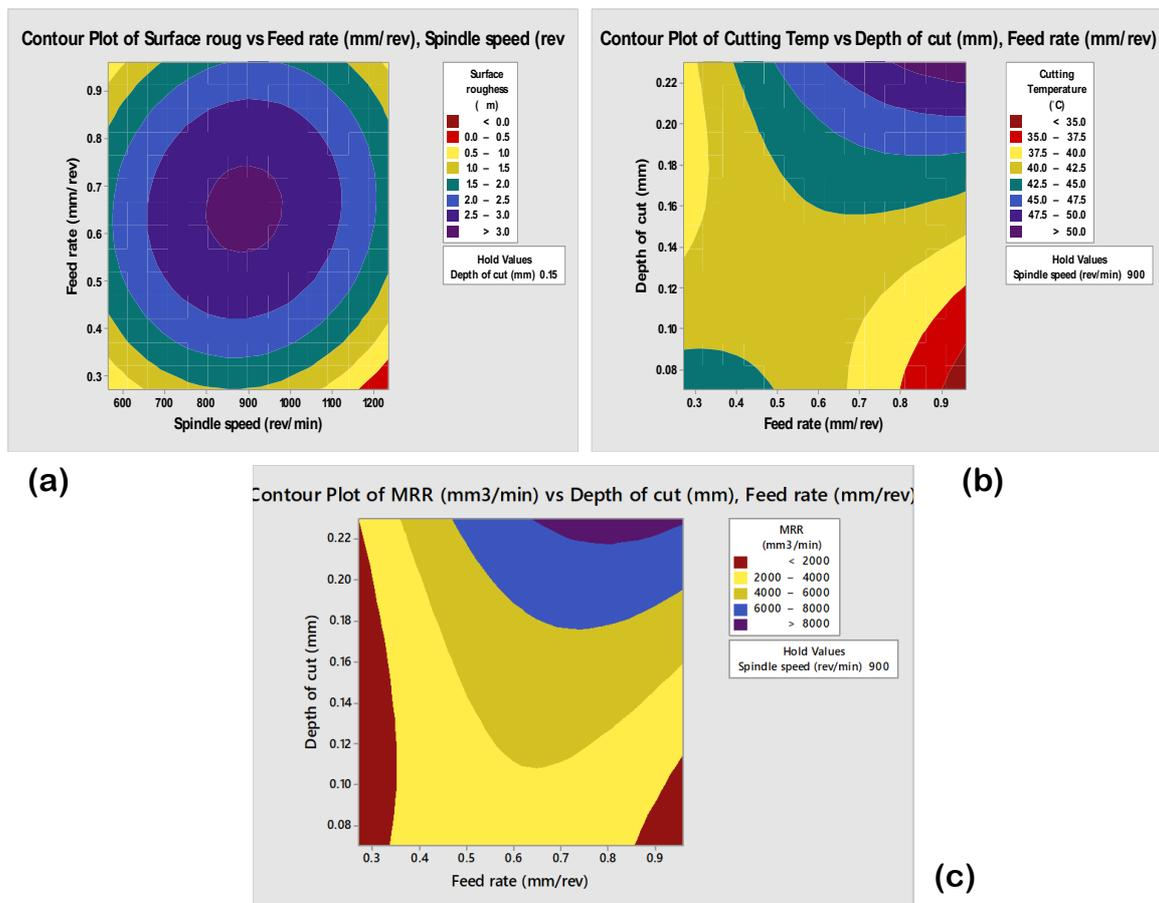
**Figure 7:** Contour plots for responses of CBCF (a) surface roughness (b) cutting temperature (c) MRR
