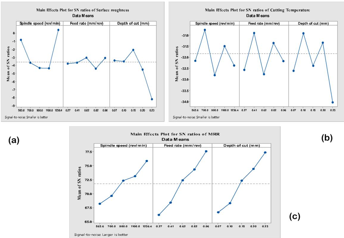
Figure 4: Main effect plots for responses of MBCF (a) Surface roughness (b) Cutting temperature (c) MRR
