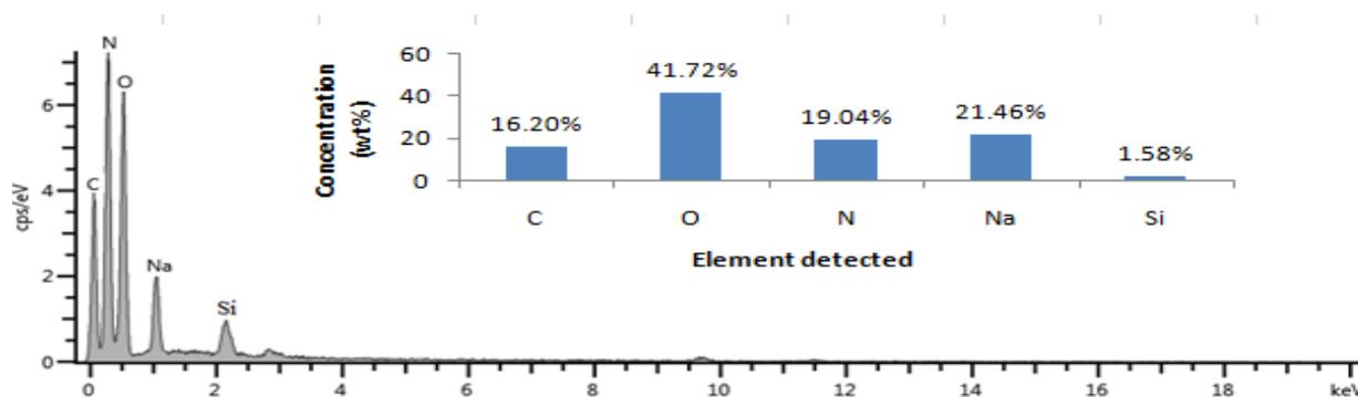
**Figure 2a:** EDS spectrum of chitosan. The inset is a histogram showing percent distribution of elements.
