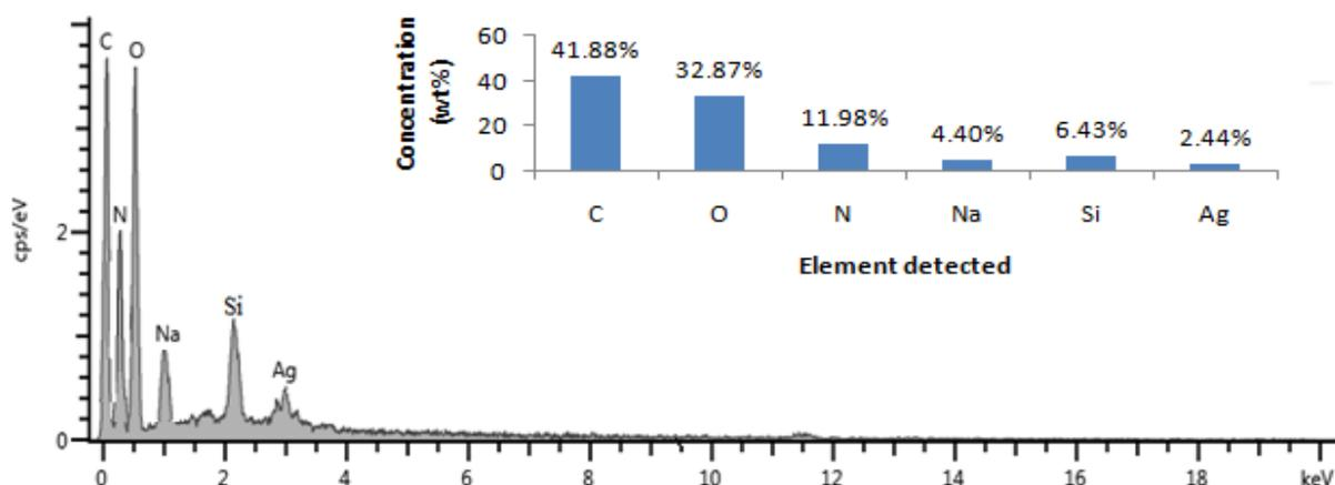
**Figure 2e:** EDS spectrum of chitosan–silver nanocomposite (COMP 2:1). The inset is a histogram showing percent distribution of elements.
