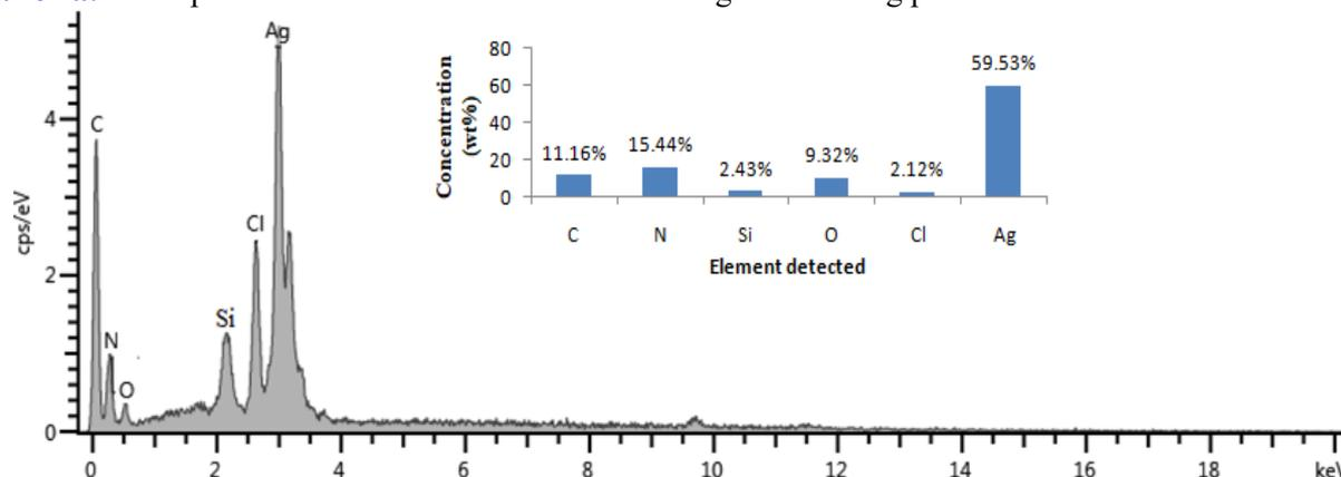
**Figure 2b:** EDS spectrum of silver nanoparticles. The inset is a histogram showing percent distribution of elements.
