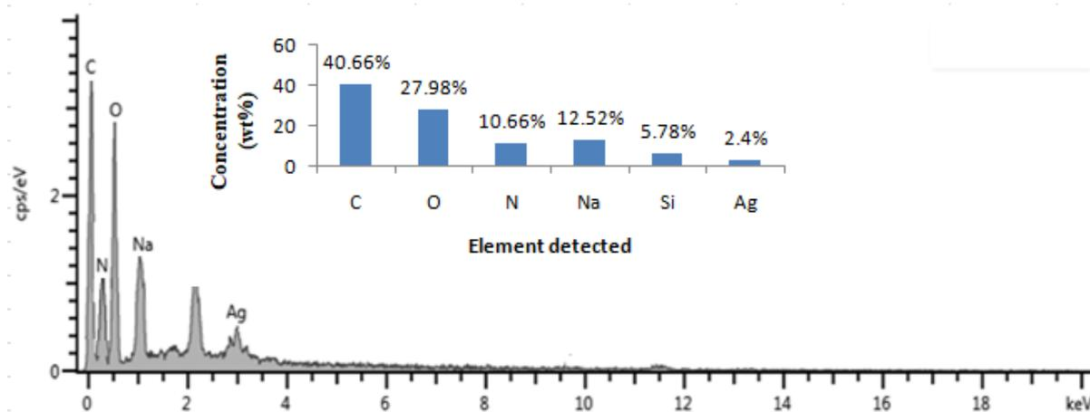
**Figure 2c:** EDS spectrum of chitosan–silver nanocomposite (COMP 1:1). The inset is a histogram showing percent distribution of elements.
