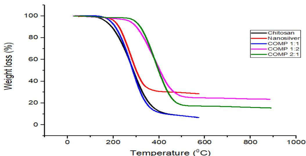
**Figure 1a:** TGA curves of the prepared chitosan, silver nanoparticles and chitosan-silver nanocomposites
