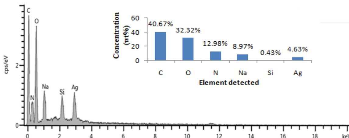
**Figure 2d:** EDS spectrum of chitosan–silver nanocomposite (COMP 1:2). The inset is a histogram showing percent distribution of elements.
