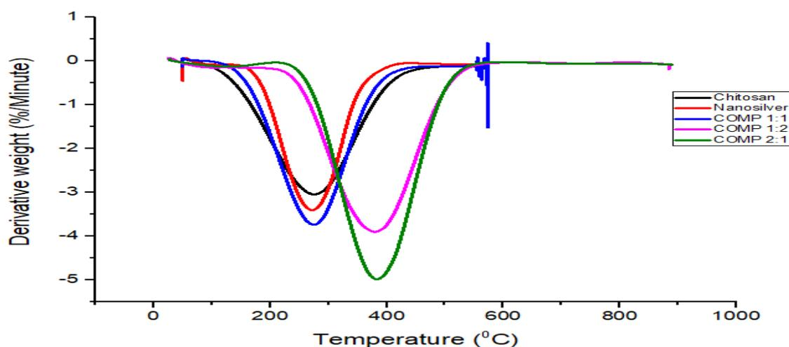
**Figure 1 b:** Thermograms of the prepared chitosan, silver nanoparticles and chitosan-silver nanocomposites
