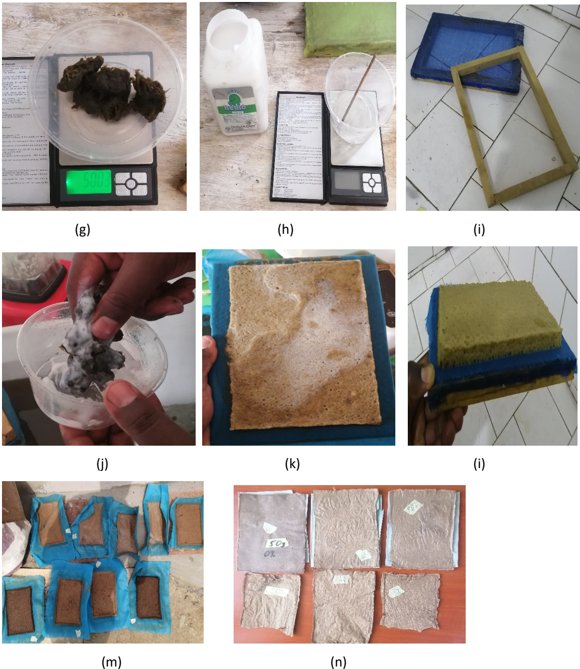
Figure 2. Process of obtaining paper from water hyacinth [Authors]
