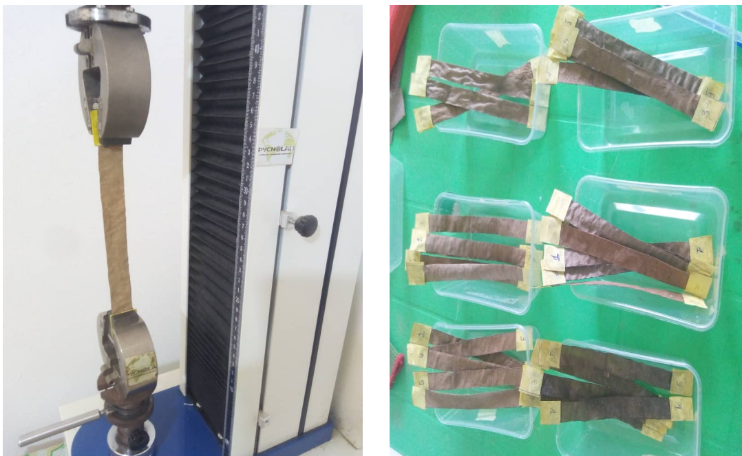
Figure 3. paperboard composites prepare to measure Mechanical properties
