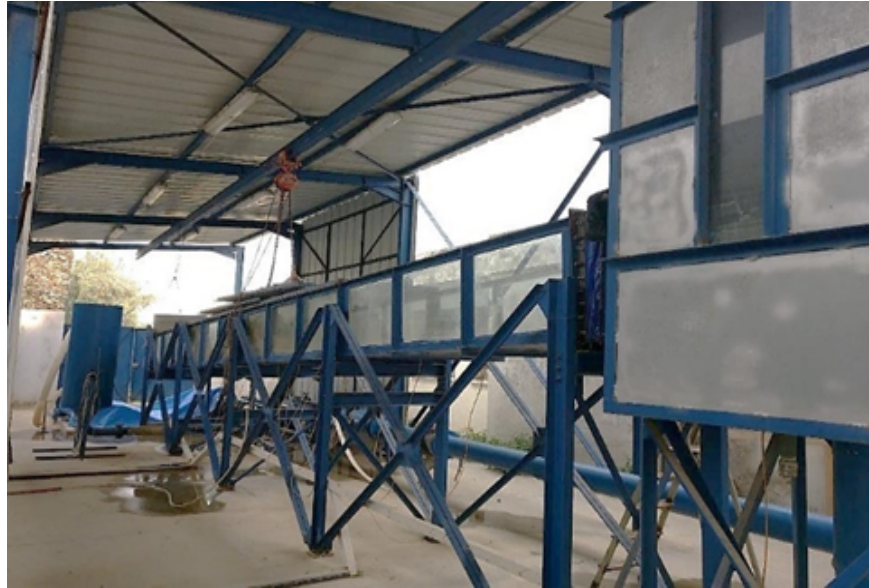
Figure 2. Experimental Setup at the INAT laboratory (Length: 10m; width: 0.8m; Hight: 0.6m)
