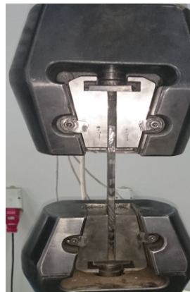
Figure 3. Experimental setup for the tensile tests
