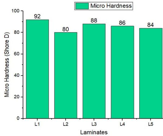
**Figure 5.** Micro- Hardness number of different laminates
