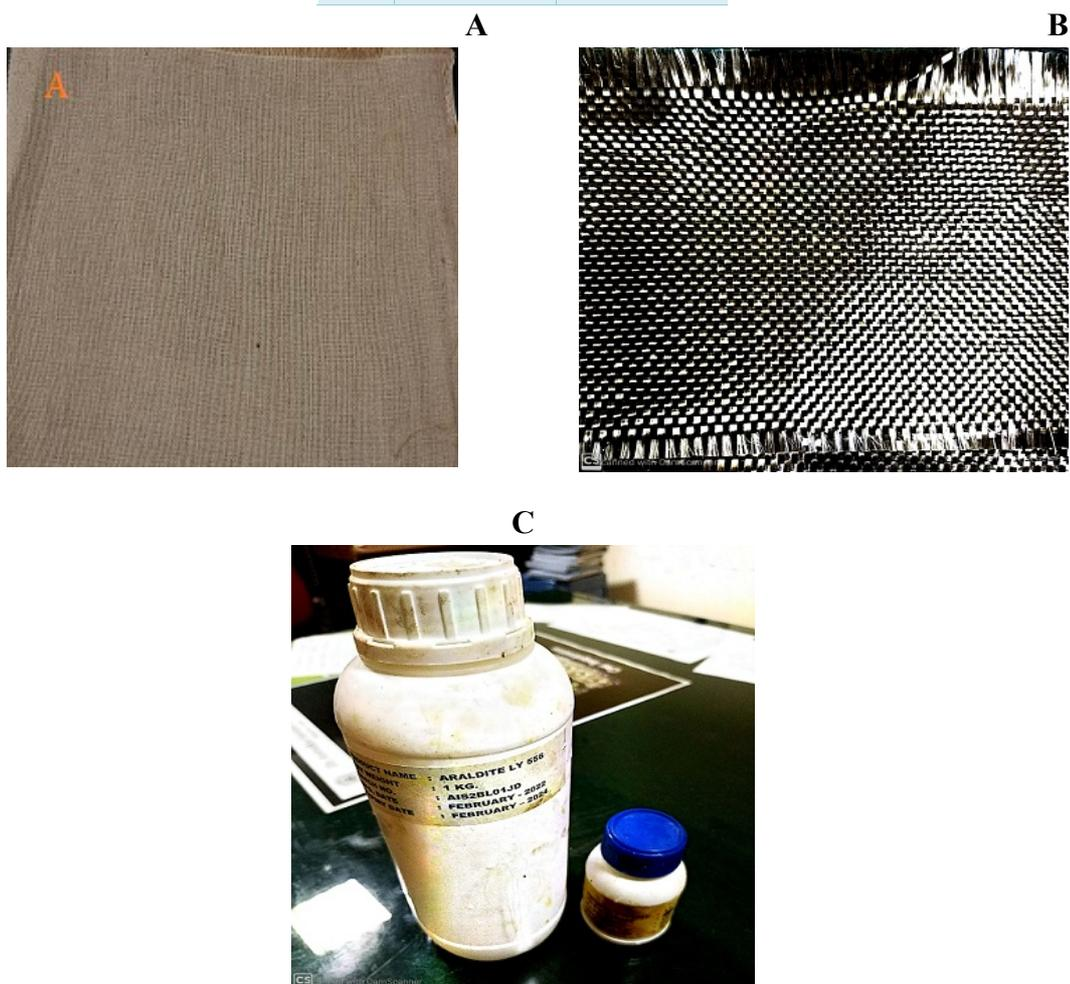
**Figure 1.** A. Ramie fabric B. Basalt Fabric C. Epoxy resin and hardener
