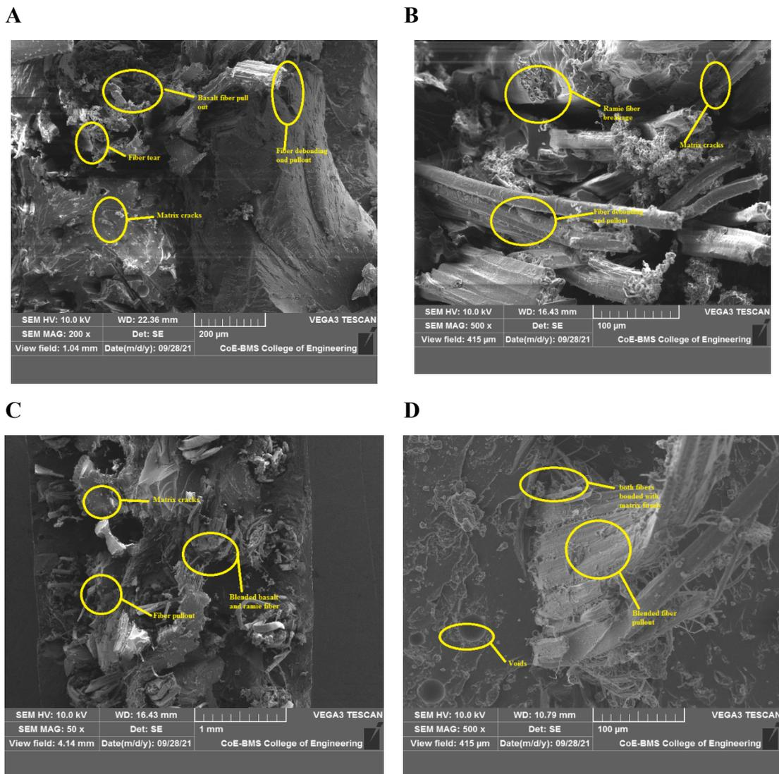
**Figure 6.** A. basalt composite B. Ramie composites C. Hybrid composites of L3 D. Hybrid composites of L4
