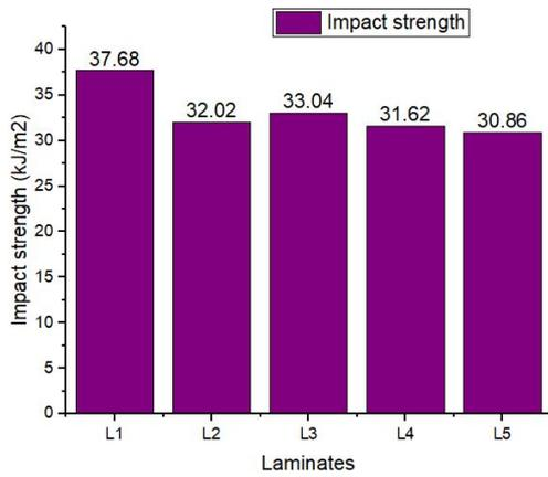
**Figure 4.** Impact strength of different laminates
