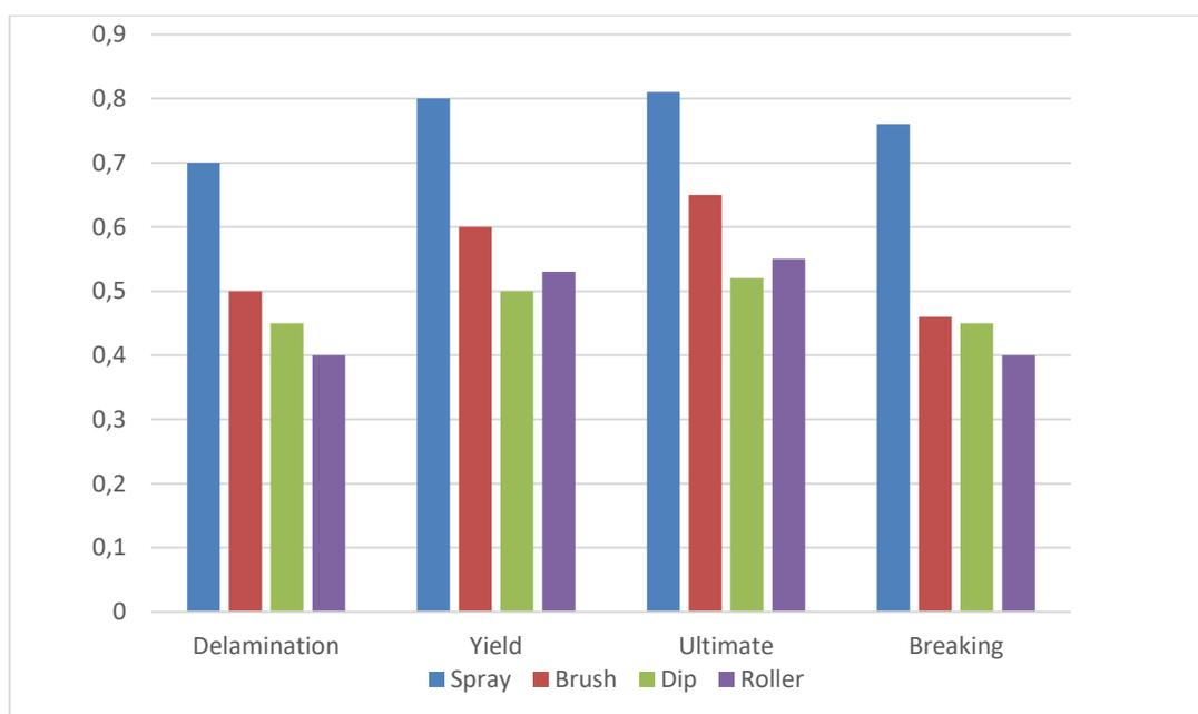
**Figure 2.** Salient features of un-notched jute-epoxy composite laminate specimens with different gel coating methods
