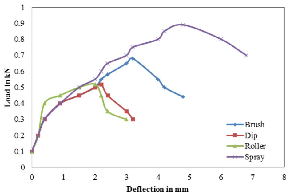
**Figure 11.** Load/Deflection for coated un-notched jute-epoxy composite laminate specimen
