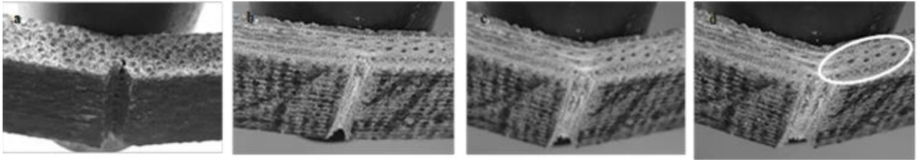
**Figure 5.** Specimen failure with notch along the laminate
