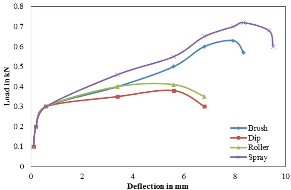
**Figure 9.** Load/Deflection for coated jute-epoxy composite laminate specimen with notch along the laminate
