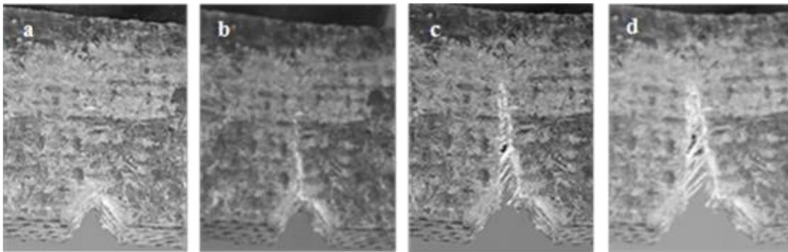
**Figure 4.** Crack growth at notch root across the laminate
