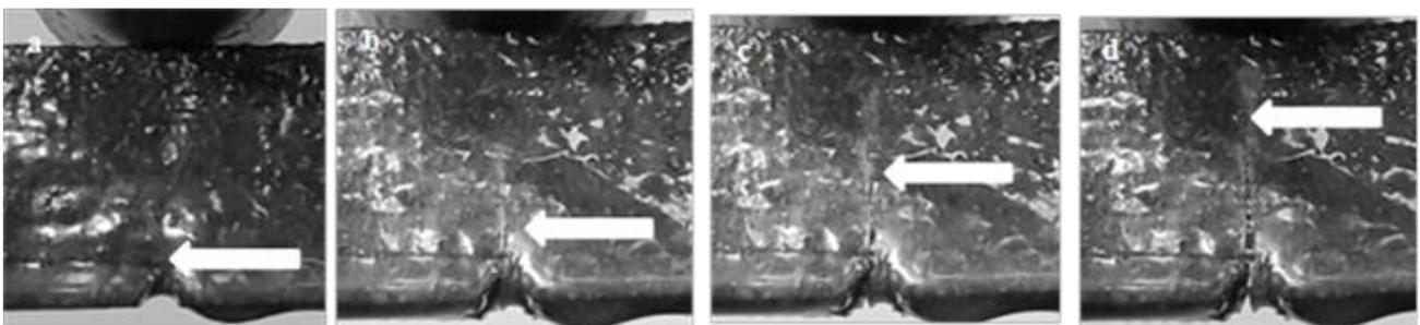
**Figure 8.** Failure in coated specimen with notch across the laminate
