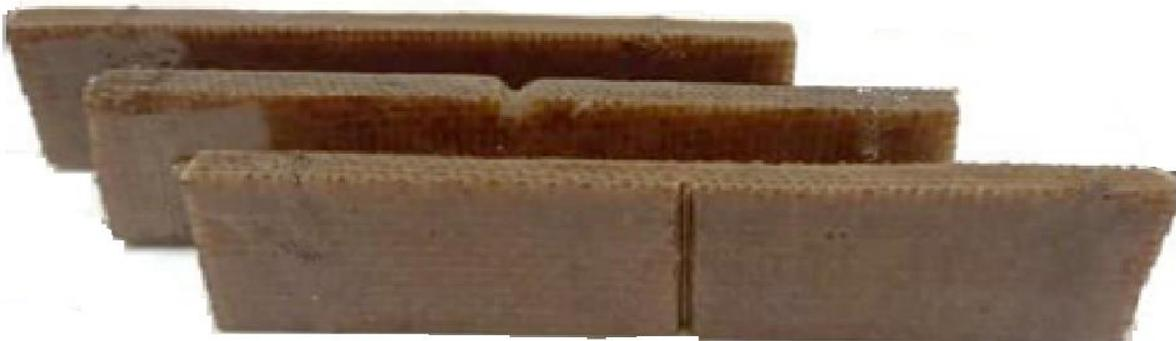
**Figure 1** Three point bending specimen as per ASTM with different notch orientation
