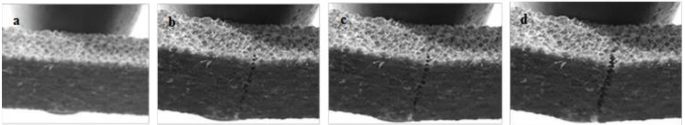
**Figure 6.** Specimen failure in un-notched specimen
