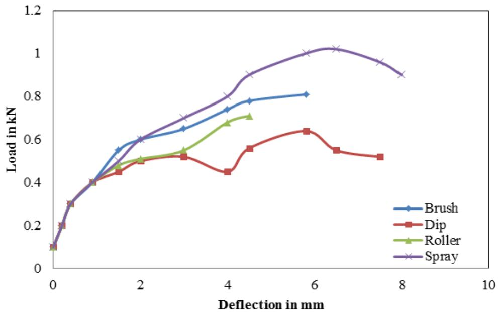
**Figure 7.** Load/Deflection for coated jute-epoxy composite laminate specimen with notch across the laminate
