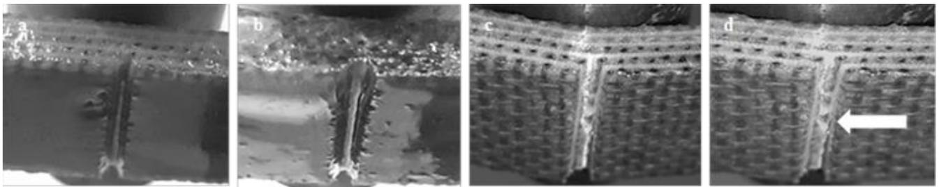
**Figure 10.** Failure in coated specimen with notch along the laminate
