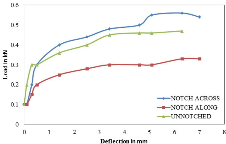
**Figure 3.** Load/Deflection for uncoated jute-epoxy composite laminate specimens with varied flaw orientation
