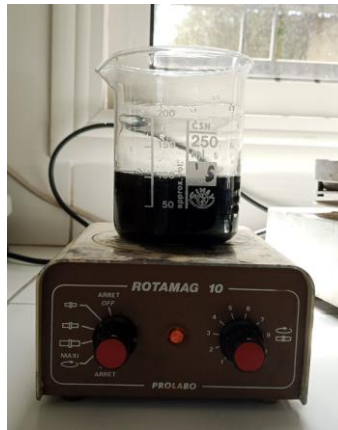
Figure 4. Chemical activation of carbon by phosphoric acid.
