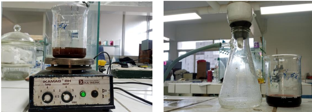
Figure 5. Chemical activation of carbon by caustic soda.
