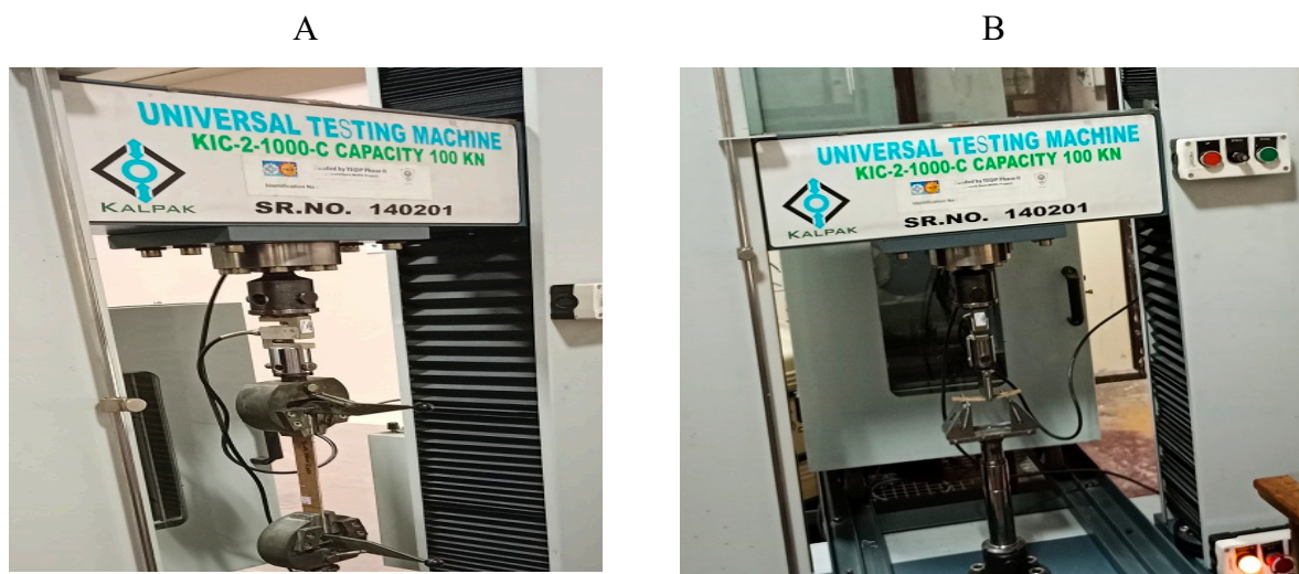
Figure 3. A. Specimen for tensile testing B. Specimen for Flexural testing
