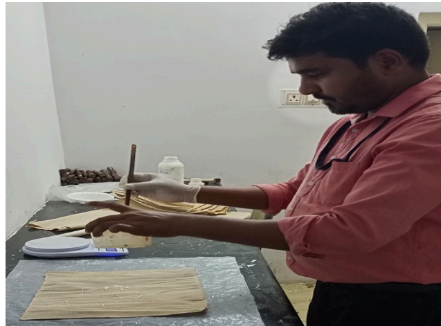
Figure 2. Hand Layup Process
