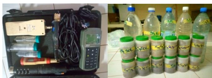
**Figure 2.** (a): Multi-parameter; (b) Sample Jars and Canisters
