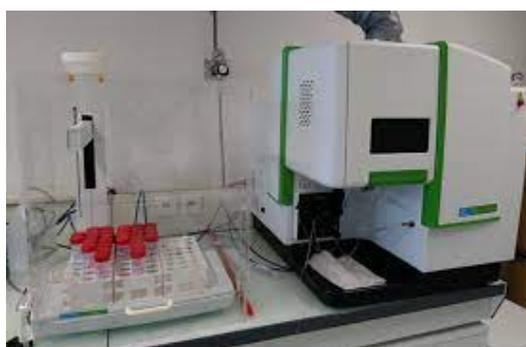
**Figure 3.** Heavy metal assay device - ICP AVIO 200
