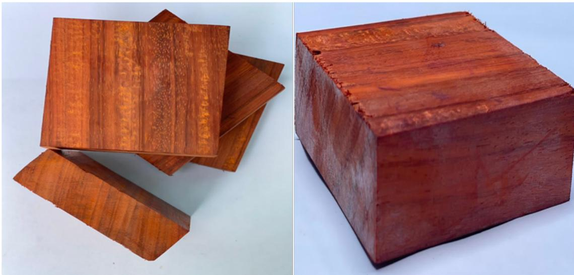
**Figure 1.** Wood samples used for the characterization of thermal properties at high temperatures
