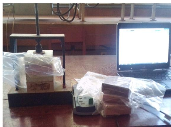
**Figure 3.** Asymmetrical hot plane experimental device
