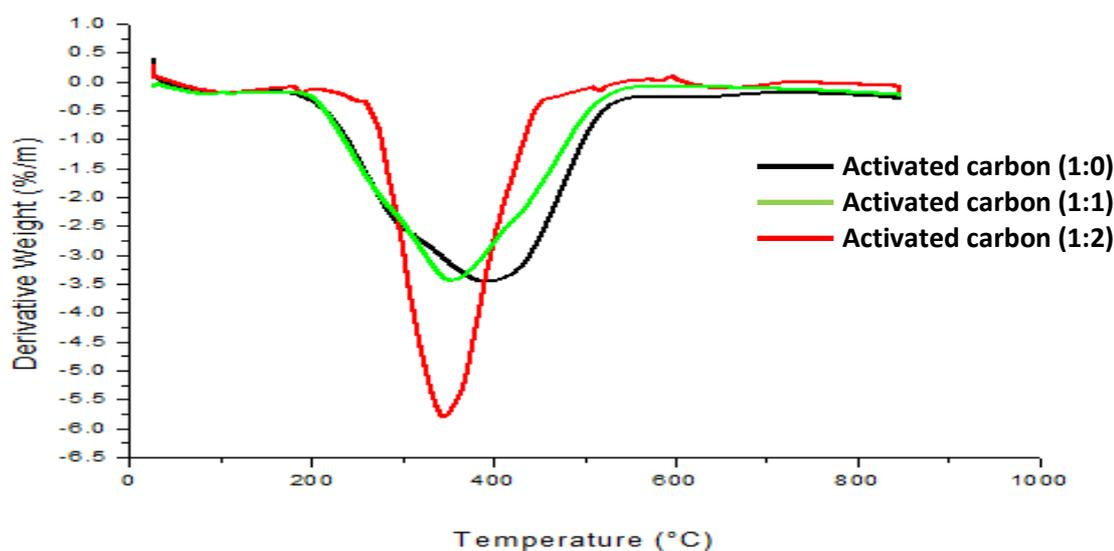
Figure b: Thermograms of the prepared activated carbons
