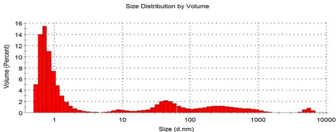
**Figure 2a:** Particle size distribution chart for the activated carbon 1:0
