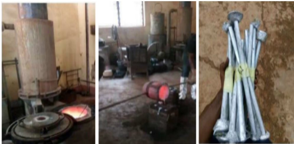
Figure 2. Showing the casting to the finished products
