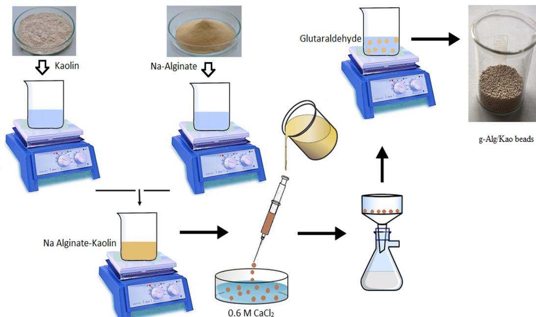
**Figure 1.** A schematic diagram presenting the preparation of g-Alg/Kao
