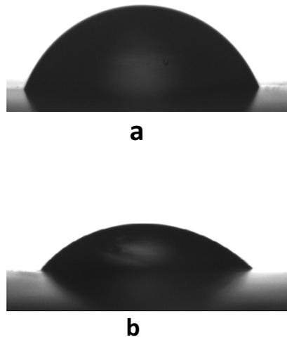
**Fig. 3.** Contact angles of pristine membrane (a), and modified membrane (b).
