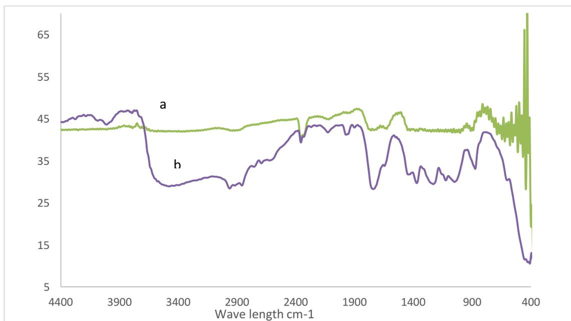
**Fig. 2:** FTIR spectra of (a) pristine CA-RO membrane and (b) modified membrane containing *Cymbopogon proximus* extract.
