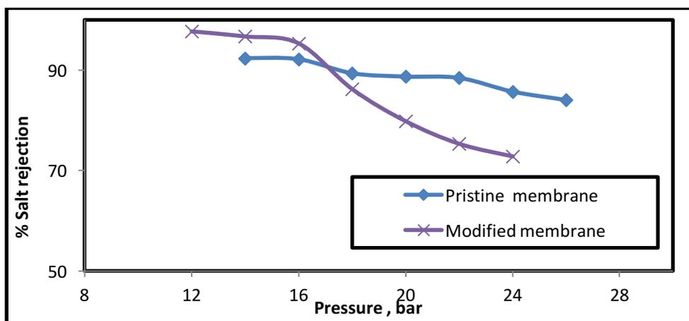
Fig 7: Variation of the percentage of salt rejection of pristine and modified membranes versus feed pressure.
