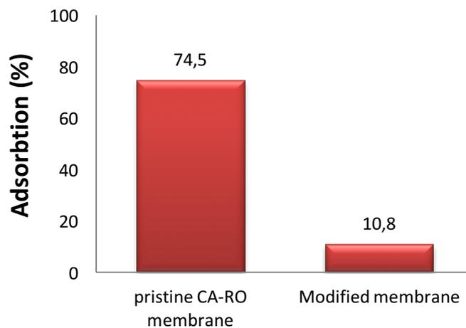
**Fig. 4.** Static adsorption of protein on pristine and modified membranes.
