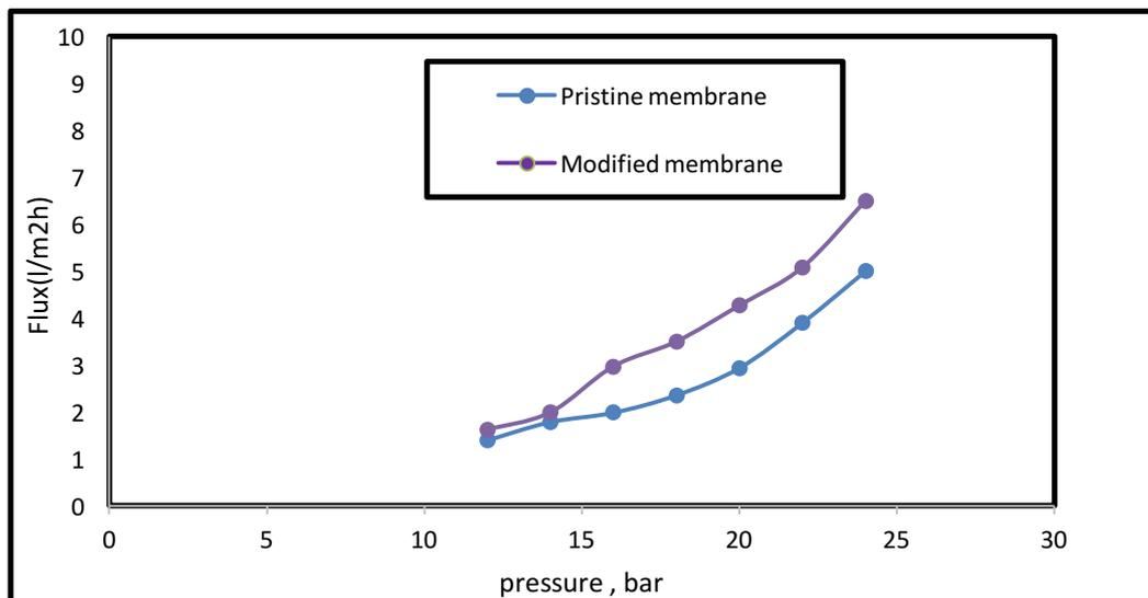
Fig. 6. Variation of permeate water flux of pristine and modified membranes versus feed pressure.
