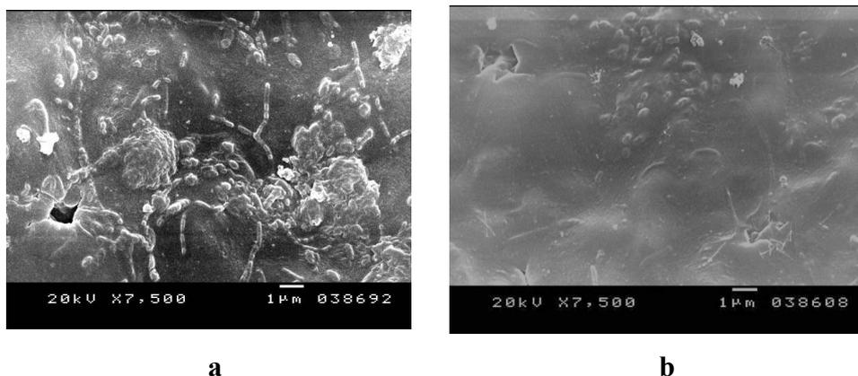
**Fig.5.** SEM photograph of pristine membrane (a) and modified membrane (b) after immersion in seawater for 15 d.
