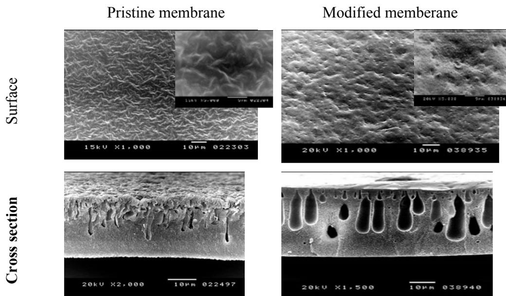
**Fig. 1.** SEM images of surface, bottom, and cross section of pristine CA-RO membrane and modified membrane containing *Cymbopogon proximus* extract.
