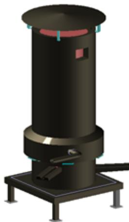
**Figure 1:** Designed pictorial view of a conventional Cupola Furnace
